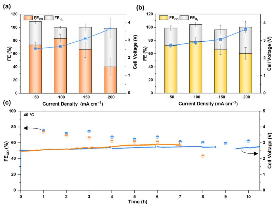
Fig. 4 FE and cell voltage profiles. (a) No  $CO_2$  purging and (b) with  $CO_2$  purging as a function of applied current densities ( $-50 \sim -200\text{ mA cm}^{-2}$ ), and (c) the long-term durability test of the Ni-SAC in a flow cell at  $-50\text{ mA cm}^{-2}$ .
