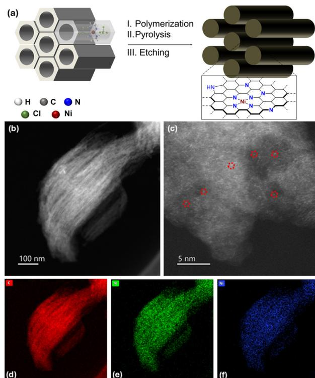
**Fig. 1** Synthesis and microscopic characterization of the Ni-SAC. (a) Schematic representation of the general synthetic method for the Ni-SAC; (b, c) aberration-corrected HAADF-STEM image; (d, e, f) EDS mapping, illustrating the spatial distributions of C (red), N (green) and Ni (blue).
