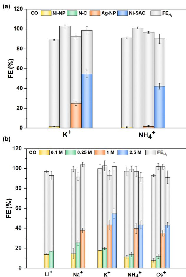
**Fig. 2** FE comparisons between different catalysts and in various cation environments. (a) FE comparison between Ni-NP, N-C, Ag-NP and Ni-SAC in 2.5 M KHCO<sub>3</sub> and NH<sub>4</sub>HCO<sub>3</sub> catholytes (carbon paper: Freudenberg H23, current density:  $-100 \text{ mA cm}^{-2}$ , temperature: RT, catalyst loading:  $1 \text{ mg cm}^{-2}$ ), and (b) FE of the Ni-SAC in bicarbonate electrolytes containing different alkali cations (concentration : 0.1 M ~ 2.5 M).
