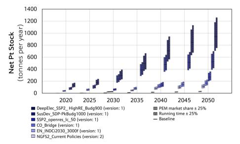
Fig. 4 Net platinum demand over six scenarios represented by a range for each scenario. The range shows the impact of ±25% to the assumed quantity of energy from hydrogen that will come from PEM fuel cells represented by a solid colour and the impact of +25% of the running hours of the fuel cell over its lifetime represented by hatched colours.
