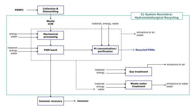
Fig. 2 System boundaries of secondary platinum from (a) current pyrometallurgical recycling route (adapted from International Platinum Group Metals Association<sup>6</sup>) and (b) potential future hydrometallurgical route.
