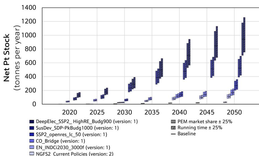
**Fig. 4** Net platinum demand over six scenarios represented by a range for each scenario. The range shows the impact of  $\pm 25\%$  to the assumed quantity of energy from hydrogen that will come from PEM fuel cells represented by a solid colour and the impact of  $\pm 25\%$  of the running hours of the fuel cell over its lifetime represented by hatched colours.
