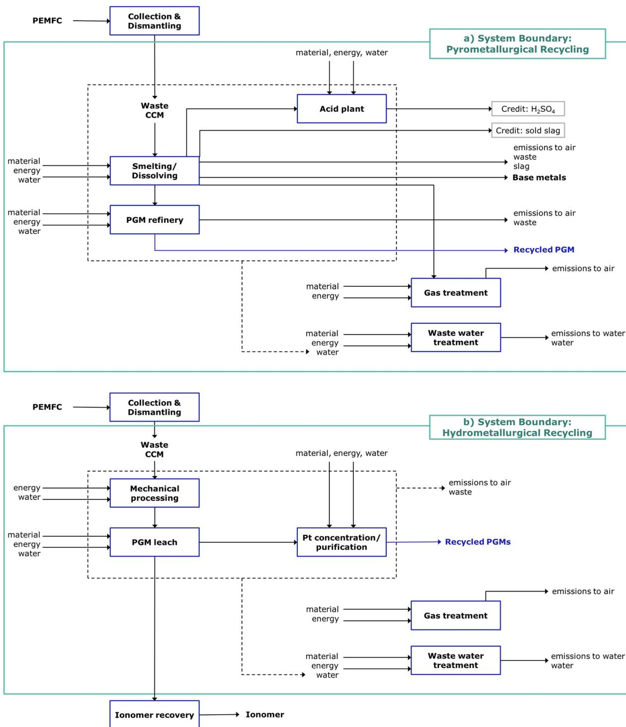
Fig. 2 System boundaries of secondary platinum from (a) current pyrometallurgical recycling route (adapted from International Platinum Group Metals Association<sup>6</sup>) and (b) potential future hydrometallurgical route.
