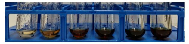
Fig. 13 Samples containing  $[C_2C_1im][OAc]$  with 15 wt% water and 5% shredded bottle PET heated at 180 °C as a function of time. Hydrolysis duration from 0.5 h (left) to 3 h (right) in 0.5 h increments.
