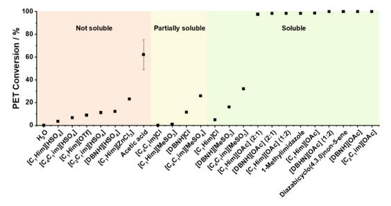
Fig. 11 PET conversion in ILs or molecular solvents at 180 °C after 3 h with 15 wt% H<sub>2</sub>O present, categorised according to solubility of 5 wt% TPA in the aqueous solvent mixtures.
