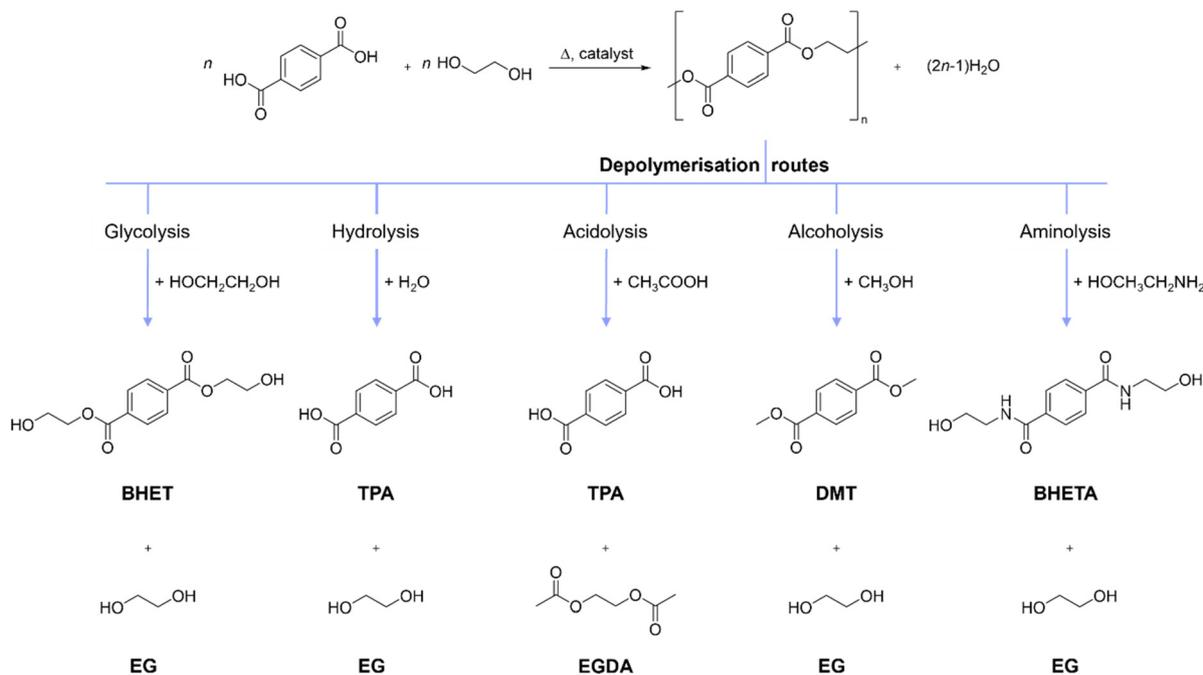
**Fig. 1** Industrial production of PET and depolymerisation routes using various nucleophiles which produce terephthalic acid, bis(2-hydroxyethyl) terephthalate, dimethyl terephthalate, bis(2-hydroxyethyl) terephthalamide, ethylene glycol (EG) or ethylene glycol diacetate (EGDA).
