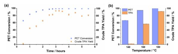
Fig. 3 PET hydrolysis in the benchmark IL,  $[C_2C_1im][OAc]$ , with 15 wt% water. (a) Conversion and isolated crude yield at 180 °C. (b) Impact of reaction temperature on PET conversion and isolated crude TPA yield at a reaction time of 3 h.
