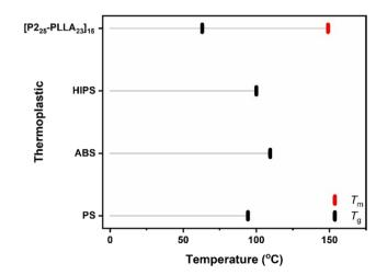
Fig. 8 Line graph showing upper temperature limits (service) for commercial polystyrene samples and lead PLLA samples from this work.
