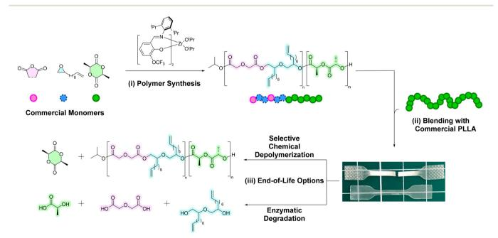
Scheme 1 The strategy for producing poly(ester-alt-ethers) used to toughen commercial, semi-crystalline PLLA. The approach in this work includes: (i) synthesis of poly(ester-alt-ether)-b-PLLA block copolymers, (ii) blending with commercial PLLA and (iii) developing chemical recycling and enzymatic degradation processes.
