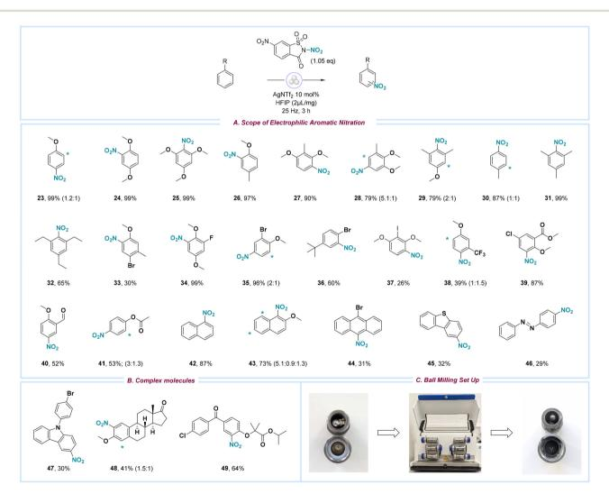
Scheme 3 (A) Substrate scope for electrophilic aromatic nitration using NN as nitrating reagent. Standard reaction conditions: 4-nitrophenethyl alcohol (0.3 mmol, 1.0 eq.), AgNTf<sub>2</sub> (10 mol%), reagent NN (1.05 eq.), HFIP (2  $\mu$ L mg<sup>-1</sup>), stainless steel jar (10 mL), stainless steel balls (3  $\times$  12 mm), 25 Hz, 3 h. (B) Scope of complex molecules. (C) Representative set-up with the Retsch Mixer Mill MM 500 vario.
