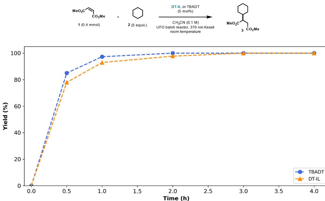
Fig. 1 Kinetic profiles for the photocatalytic Giese-type coupling of cyclohexane and dimethyl maleate comparing TBADT and DT-IL as photocatalysts. Reaction conditions: TBADT or DT-IL (5 mol%), dimethyl maleate (0.4 mmol), cyclohexane (2.0 mmol), acetonitrile (0.1 M), UFO batch photochemical reactor,<sup>16</sup> 370 nm Kessil LED (44 Watt).
