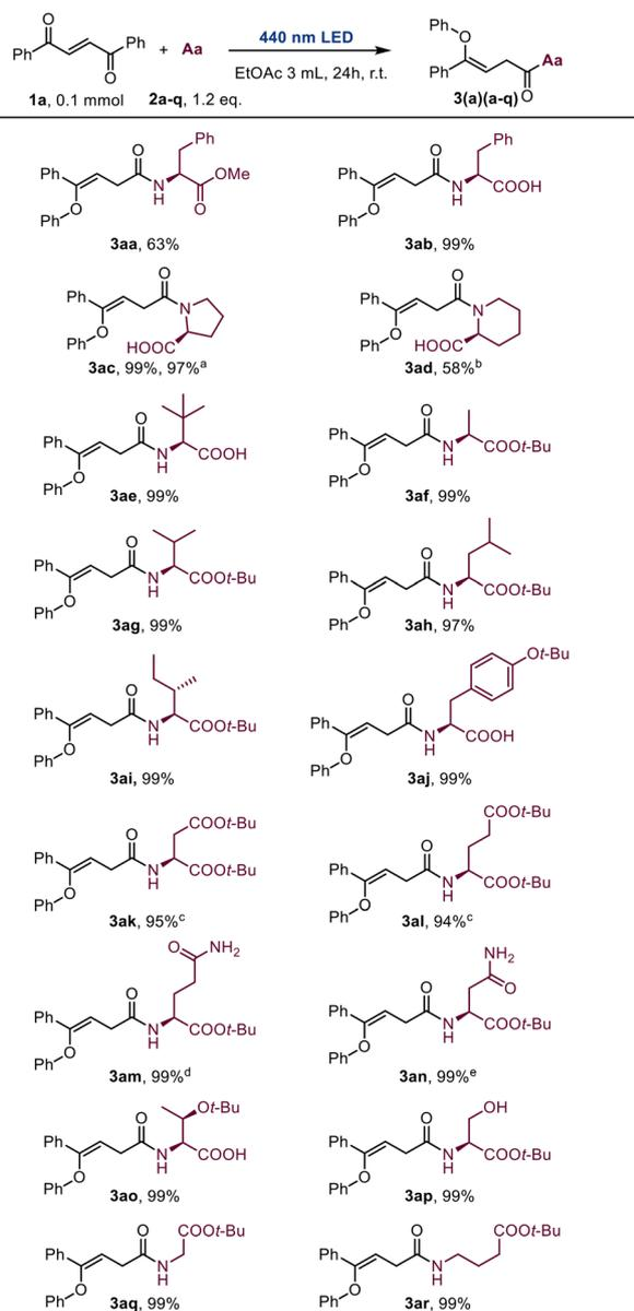
**Scheme 2** Substrate scope of amino acids run under optimal conditions of Table 1. <sup>a</sup>Yield from the upscaling experiment. <sup>b</sup>Reaction performed at 0.125 mmol scale. <sup>c</sup>1.05 equivalents of nucleophile. <sup>d</sup>2 equivalents of nucleophile. <sup>e</sup>4 equivalents of nucleophile.
