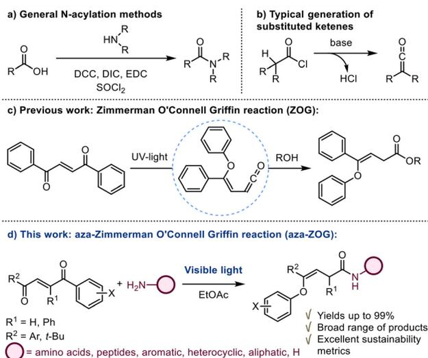
**Scheme 1** (a) *N*-Acylation by using coupling reagents on carboxylic acids. (b) Typical generation strategy of substituted ketenes. (c) Previous work: ZOG reaction generating ketenes solely by UV irradiation. (d) This work: development of the visible-light-driven aza-ZOG reaction.
