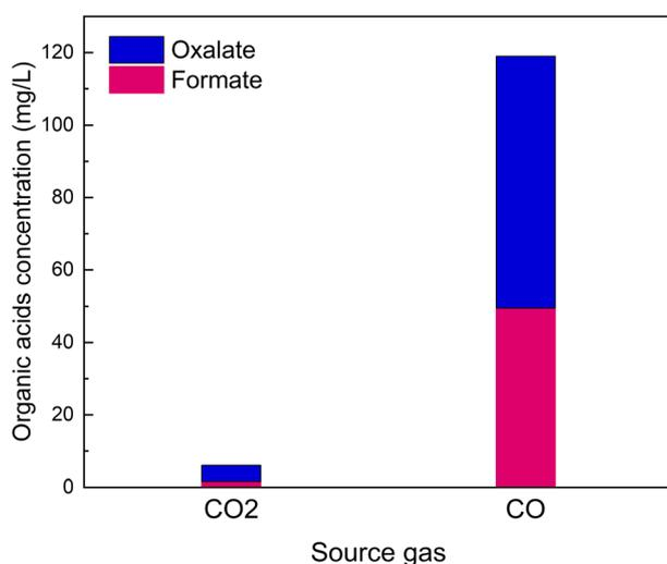
**Fig. 2** CO process gas produced more organic acids than CO<sub>2</sub>. Mass concentration of oxalate (blue) and formate (magenta) as measured by ion chromatography for CO<sub>2</sub> and CO process gas. The initial electrolyte composition was 1 mM NaOH.
