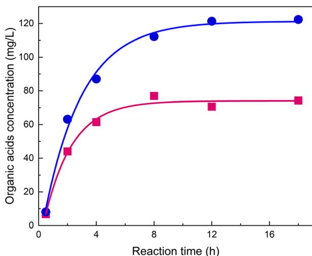
**Fig. 5** Steady state of organic acid concentration indicates these species are intermediates in the overall water gas shift reaction. The initial electrolyte concentration was 1 mM NaOH. Mass concentration of oxalate as measured by ion chromatography for different reaction times at 1 mM NaOH.
