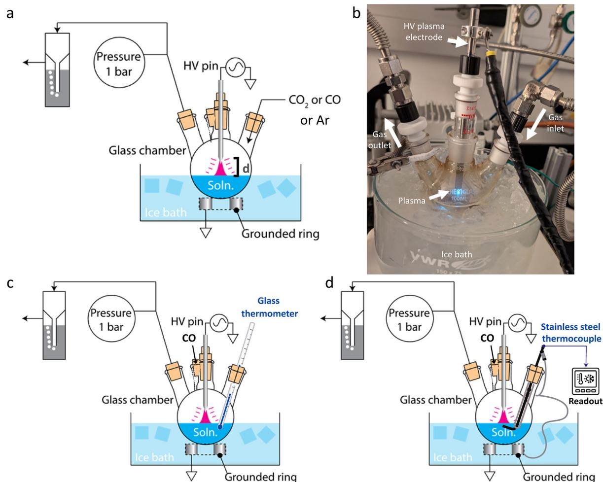
**Fig. 1** Plasma–liquid reaction experimental schematic. (a) Schematic representation of major components and (b) digital photograph of the experimental setup during non-thermal atmospheric pressure plasma–liquid reaction for organic acids synthesis. Schematic representation of modified setup for temperature measurements (c) far away ( $\sim 17$  mm distance and 10 mm depth) from the plasma–liquid reaction region and (d) close to ( $\sim 5$  mm depth) the plasma–liquid reaction region.
