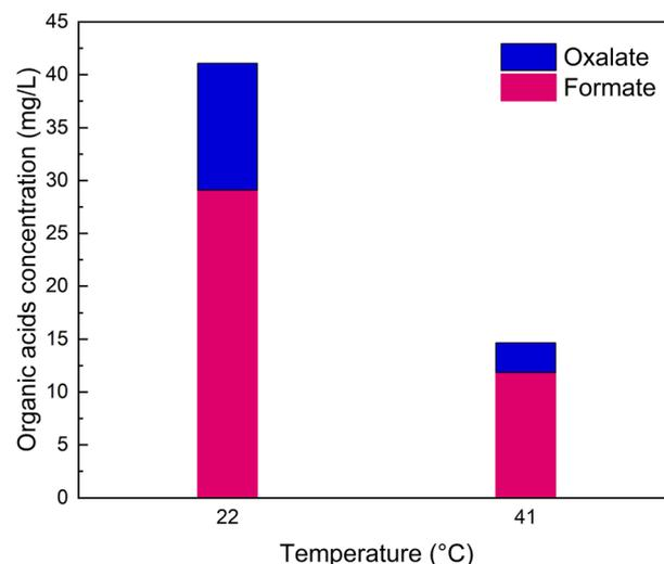
**Fig. 3** A higher yield of organic acids was obtained at lower solution temperature. Mass concentration of oxalate (blue) and formate (magenta) as measured by ion chromatography for reactions at lower (22 ± 2 °C) and higher (41 ± 2 °C) temperatures. The initial electrolyte composition was 10 mM NaOH.
