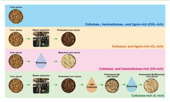
Fig. 1 The overall procedure for preparing different types of lignocellulosic material
