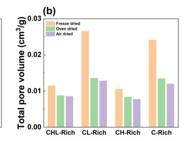
Fig. 5 BET surface area (a) and total pore volume (b) of CHL-rich, CL-rich, CH-rich and C-rich substrates after various drying methods, determined by nitrogen adsorption analysis.
