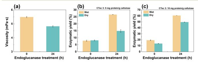
Fig. 7 Effect of 24 h endoglucase treatment on pulp viscosity (a) and cellulose hydrolysis yield at enzyme loadings of 5 mg (b) and 10 mg (c) per g cellulose. The hydrolysis was conducted in a pH 4.8 buffer at 2% solids loading.
