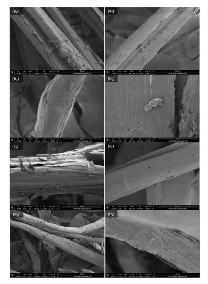
Morphology of freeze-dried (a) CHL-rich, (b) CL-rich, (c) CH-rich and (d) C-rich substrates determined by SEM microscopy.
