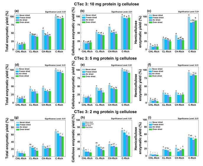
Fig. 6 72 h enzymatic hydrolysis yields of CHL-rich, CL-rich, CH-rich and C-rich substrates at enzyme loadings of 10 (a–c), 5 (d–f), and 2 (g–i) mg  $g^{-1}$  cellulose. The hydrolysis was conducted in a pH 4.8 buffer at 2% solids loading.
