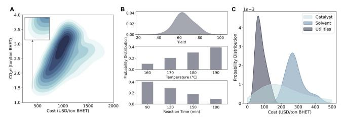
Fig. 4 Process performance analysis. (A) Distribution plot of  $CO_2e$  and cost values for the top  $10^5$  performance cases from high throughput analysis from PET bottles shredded to 5 mm. (B) Probability distribution plots for yield, temperature, and reaction time of the top  $10^4$  performance cases. (C) Probability distribution plots of cost breakdown of catalyst, solvent, and utilities of the top  $10^4$  performance cases.
