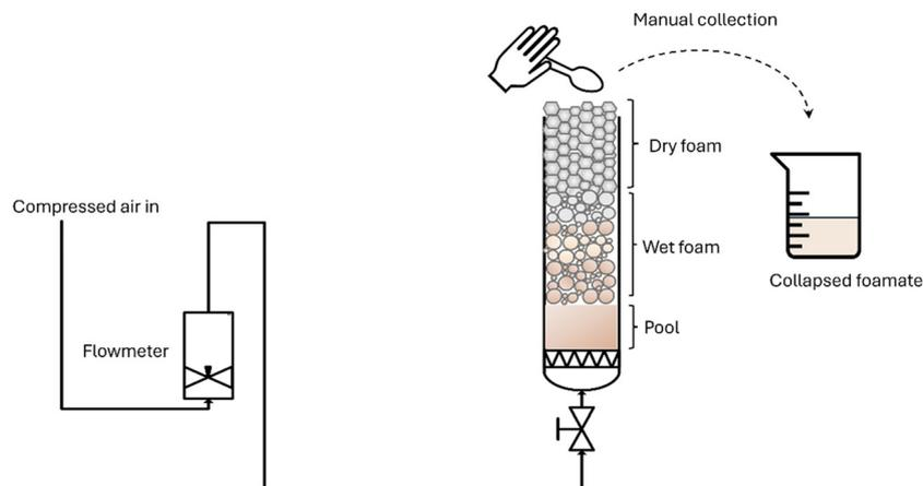
**Fig. 2** Foam fractionation setup used for the purification of surfactant mixtures.
