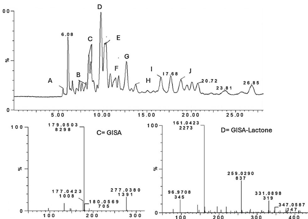
**Fig. 3** UPLC MS chromatogram and spectrum of HA mixture from MCC. A =  $(C_xH_yO_z)_{176}$ , B = glycolic acid, C = GISA, D = GISA-lactone, E =  $(C_xH_yO_z)_{178}$ , lactic acid + formic acid, F = acetic acid + formic acid, G = 2,5-DHPA, H =  $(C_xH_yO_z)_{192}$ , I = 2-HGA, and J = 2-HBA. The other spectra are available in ESI Fig. S1.†
