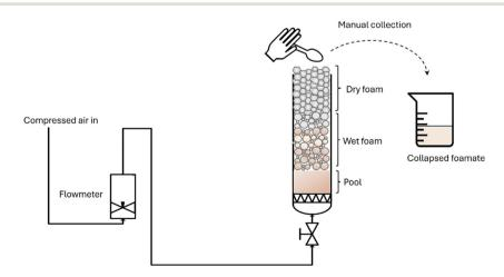
Fig. 2 Foam fractionation setup used for the purification of surfactant mixtures.
