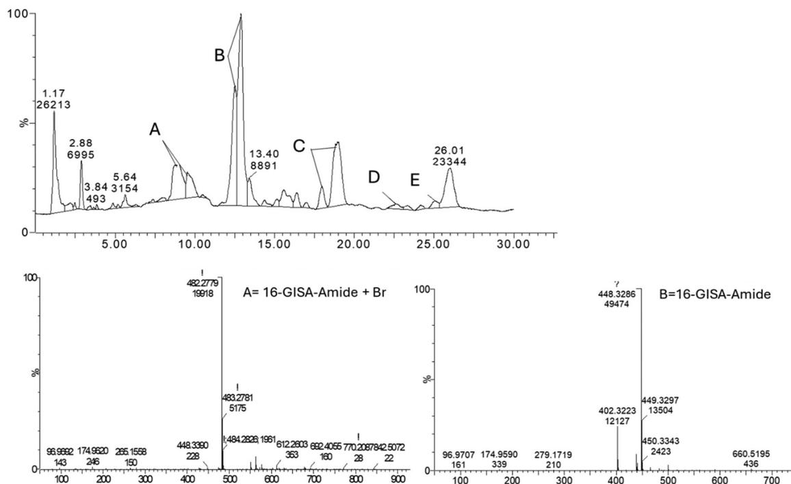
**Fig. 5** UPLC-MS chromatogram and mass spectra for reaction MCC\_C16\_PM. A = 16-GISA-Amide + Br, B = 16-GISA-Amide, C = 16-(C<sub>x</sub>H<sub>y</sub>O<sub>2</sub>)<sub>178</sub>-Amide, D = 16-HGA-Amide, and E = 16-(C<sub>x</sub>H<sub>y</sub>O<sub>2</sub>)<sub>192</sub>-Amide. The spectra for the other compounds can be seen in ESI Fig. S4.†
