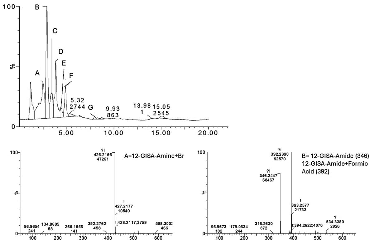
**Fig. 4** UPLC–MS chromatogram and mass spectra for reaction MCC\_C12\_PM. A = 12-GISA-Amide + Br, B = 12-GISA-Amide + formic acid, C = 12-(C<sub>x</sub>H<sub>y</sub>O<sub>z</sub>)<sub>176</sub>-Amide + formic acid, D = 12-(C<sub>x</sub>H<sub>y</sub>O<sub>z</sub>)<sub>178</sub>-Amide, E = 12-2-HGA-Amide, F = 12-(C<sub>x</sub>H<sub>y</sub>O<sub>z</sub>)<sub>192</sub>-Amide, and G = 12-lactamide. The spectra for the other compounds can be seen in ESI Fig. S2.†
