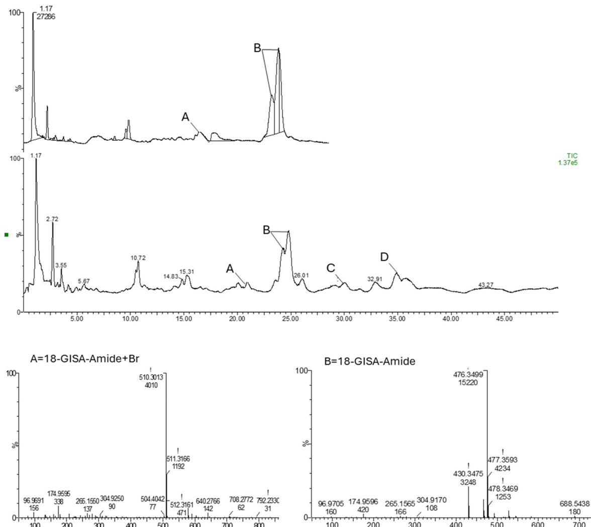
Fig. 6 Chromatogram and mass spectra for reactions of MCC<sub>18</sub>\_PM (top) and ZFS<sub>18</sub>\_PM (bottom). A = 18-GISA-Amide + Br, B = 18-GISA-Amide, C = 18-HGA-Amide, and D = 18-(C<sub>x</sub>H<sub>y</sub>O<sub>z</sub>)<sub>178</sub>-Amide. The spectra for the other compounds can be seen in ESI Fig. S6.†
