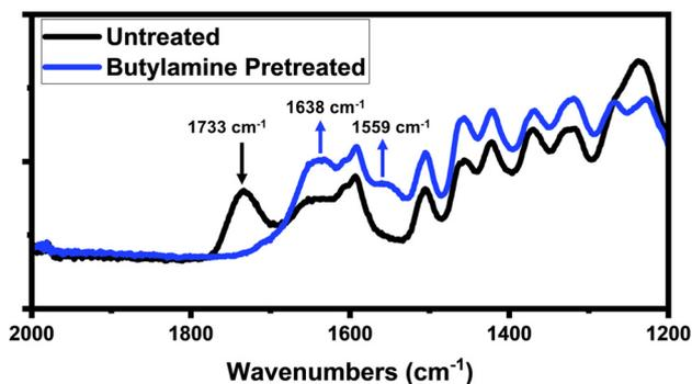
**Fig. 6** ATR-FTIR of untreated (black) and butylamine pretreated (blue) hybrid poplar samples showcasing the loss of the 1733  $\text{cm}^{-1}$  ester stretching peak in the untreated biomass, and the appearance modes at 1638  $\text{cm}^{-1}$  and 1559  $\text{cm}^{-1}$  which are assigned to amide C=O stretching and N–H bending respectively.
