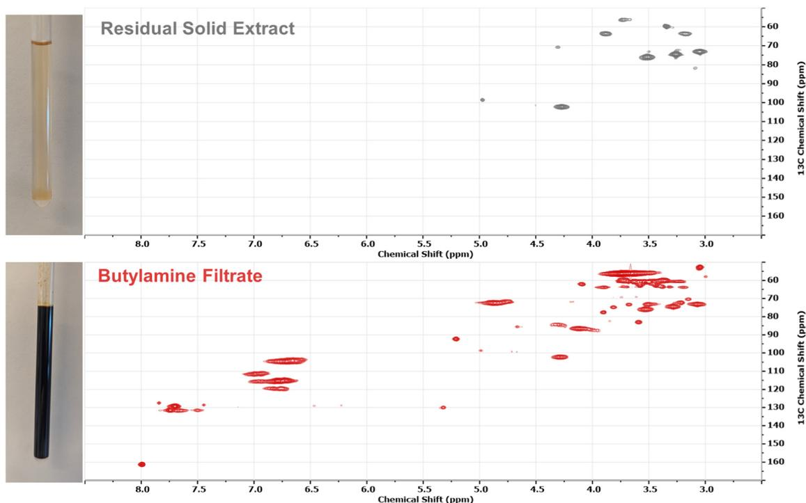
Fig. 5  $^1\text{H}$ - $^{13}\text{C}$  HSQC spectra taken in DMSO- $d_6$  of the residual solid resulting from press filtering the wet pretreatment slurry (top, grey) and the contents of the butylamine filtrate (bottom, red).
