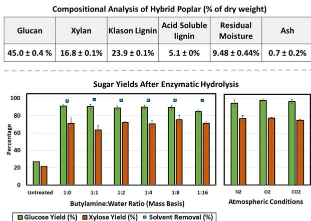
**Fig. 1** The NREL compositional analysis of the hybrid poplar sample used in this study reported in percentages of the total dry-weight of the biomass (top) and the recovered sugar yields achieved following pretreatment and enzymatic hydrolysis of hybrid poplar with varying pretreatment conditions (bottom).
