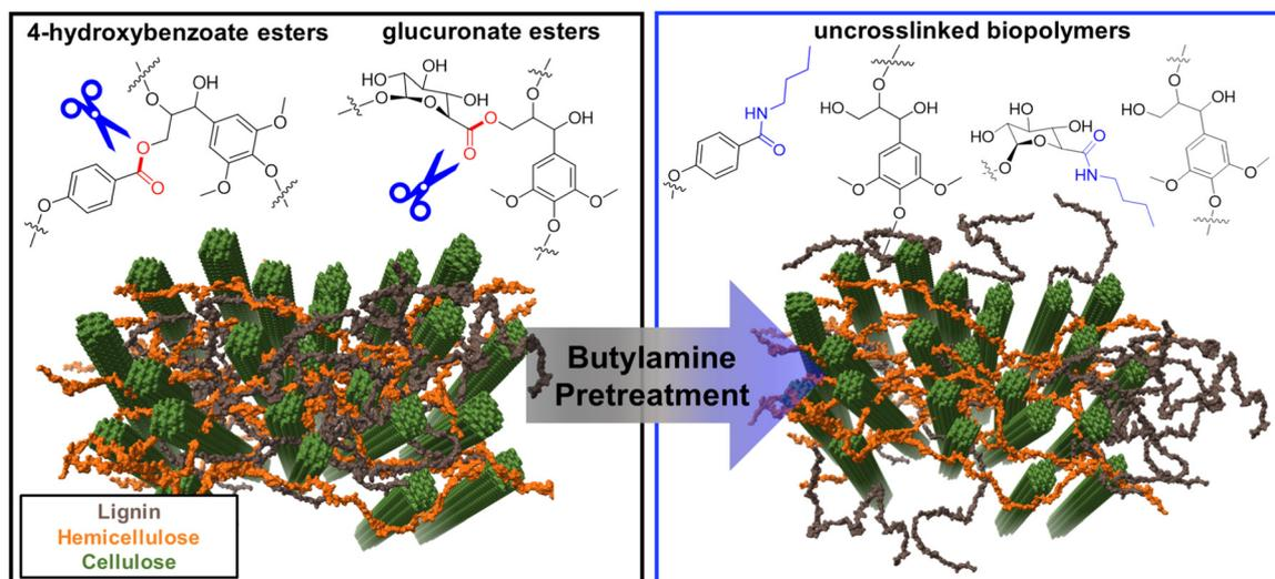
**Scheme 2** Diagram of proposed mechanism of butylamine pretreatment, showing pHB and glucuronate ester cross-linkages (left) and the cleaved amidation products (right). Below shows the proposed structural changes to lignocellulose after the lignin (grey) has been released from the interconnected structure of cellulose (green) and hemicellulose (orange).
