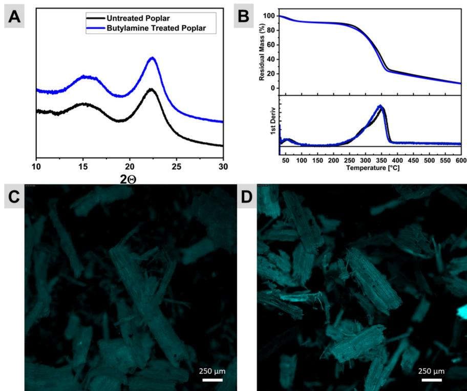
**Fig. 2** pXRD spectra (A) of untreated (black) and butylamine pretreated (blue) hybrid poplar samples, TGA (B) of untreated (black) and butylamine pretreated (blue) hybrid poplar samples, and fixed-contrast fluorescence microscopy images of untreated (C) and pretreated (D) milled particles of hybrid poplar.
