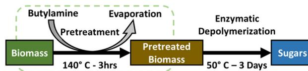
**Scheme 1** Schematic of the in-and-out pretreatment process explored within this work. The process involves an initial pretreatment step with butylamine at elevated temperature, followed by evaporative drying to yield a dry solid which is efficiently digested by a cellulase/hemicellulase enzyme cocktail to monomeric sugars.
