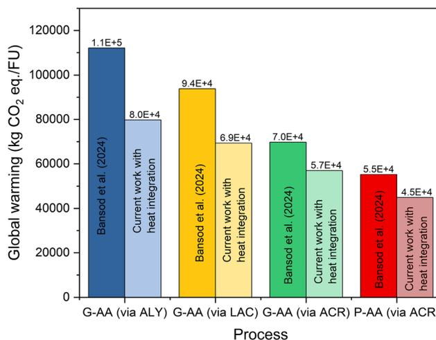
Fig. 14 Comparison of global warming potential between the previous LCA study (Bansod *et al.*, 2024)<sup>36</sup> and the current work with heat integration for the four acrylic acid production processes.
