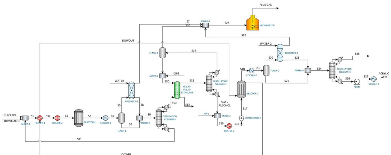
**Fig. 2** Process flow diagram for the G-AA (via ALY) process.
