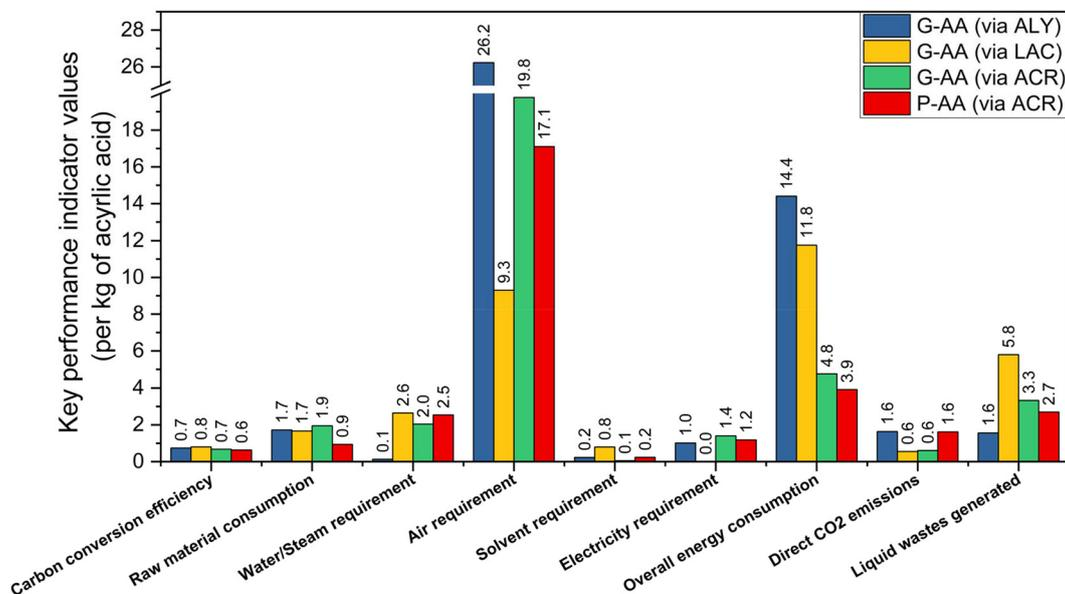
Fig. 8 Process performance indicators per kg of acrylic acid produced by the four acrylic acid production pathways. The RM, WS, AR, SR, and LW values are in kg kg<sup>-1</sup> units, whereas the ER and OER values are in kWh kg<sup>-1</sup> units.
