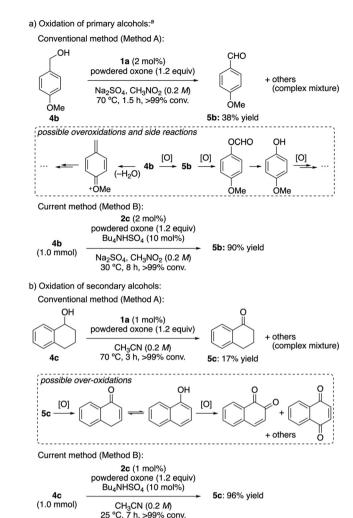
Scheme 4 Comparison of conventional and current oxidation methods: representative examples.  $^a$  Anhydrous  $Na_2SO_4$  was used as a desiccant in both the conventional and current oxidation methods to prevent aldehyde hydration to hemiacetals during the oxidation of the primary alcohols.  $^{6a}$
