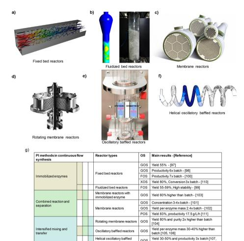
Fig. 18 Process intensification strategies for the synthesis of prebiotics. (a) Fixed bed reactors, (b) Fluidized bed reactors, (c) Membrane reactors, (d) Rotating membrane reactors, (e) Oscilatory buffle reactorz, (f) Helical oscillatory baffled reactors, (g) Table containing the processes identification results in prebiotic molecules production. Figures were adapted from ref. 179, 181, 183, 186–189.
