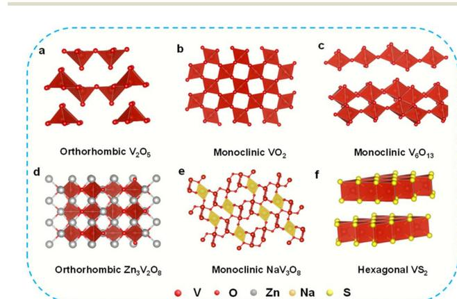
Fig. 2 Crystal structure of V<sub>2</sub>O<sub>5</sub>, VO<sub>2</sub>, V<sub>6</sub>O<sub>13</sub>, Zn<sub>3</sub>V<sub>2</sub>O<sub>8</sub>, NaV<sub>3</sub>O<sub>8</sub>, VS<sub>2</sub>.
