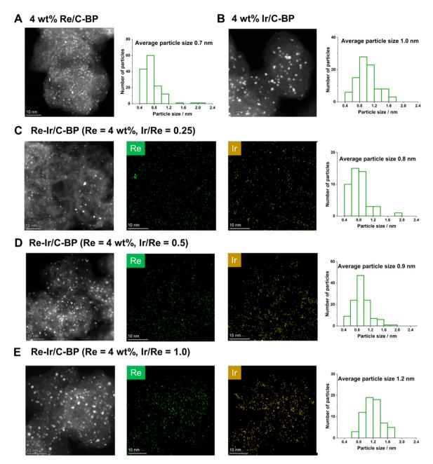
Fig. 6 HAADF-STEM images and elemental mapping of catalysts after reduction (H<sub>2</sub>, 773 K) + passivation: (A) Re/C-BP (Re 4 wt%); (B) Ir/C-BP (Ir 4 wt%); (C) Re-Ir/C-BP (Re 4 wt%, Ir/Re = 0.25); (D) Re-Ir/C-BP (Re 4 wt%, Ir/Re = 1.0).
