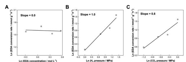
Fig. 7 Double logarithmic plots of EDA conversion rate as a function of (A) concentration of EDA, (B) partial pressure of  $H_2$ , and (C) partial pressure o
