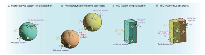
Fig. 5 Schematic representation of photocatalytic and photoelectrocatalytic (PEC) systems involving one or two light absorbers. Important differences between the two types of system include (i) a dispersed vs. monolithic architecture and (ii) charge transport through diffusion (J<sub>dif</sub>) vs. drift  $(J_{drift})$  currents.
