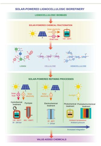
Fig. 2 Illustration of possible approaches to implement solar-powered processes in lignocellulose biorefineries for the production of valueadded chemicals from raw biomass.
