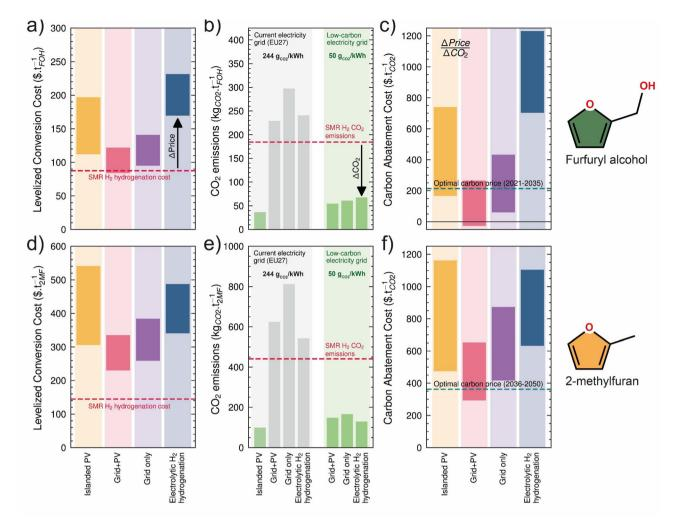
Fig. 10 Levelized conversion cost of furfural to FOH (a) and 2MF (d) compared with SMR H<sub>2</sub> hydrogenation. CO<sub>2</sub> emissions associated with ECH when electricity originates from current grid electricity (EU27) or low-carbon grid in the case of FOH (b) or 2MF (e) synthesis. CO<sub>2</sub> abatement costs of switching thermocatalytic hydrogenation of furfural to ECH of furfural for cases 1, 2, 3 and 4 in the case of FOH (c) and 2MF synthesis (f).
