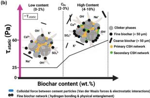
Fig. 4 Yield stress analysis of fiber cement slurry as a function of biochar content. (a) Variation of  $\dot{\tau}_{\rm static}$  &  $\dot{\tau}_{\rm dynamic}$  and  $\dot{\tau}_{\rm static}/\tau_{\rm dynamic}$ . (b) Proposed mechanism of  $\dot{\tau}_{\rm static}$  evolution with biochar. Note that Ca²+, Na+, K+, and OH $^-$  depicted in the figure represents the ions present in the cement paste pore solution.
