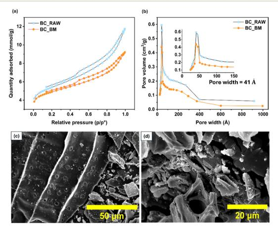
Fig. 2 Pore characterization and visualization of biochar. (a)  $N_2$  adsorption—desorption isotherms and (b) BJH pore size distribution of biochar before (BC\_RAW) and after ball milling (BC\_BM). (c-d) Representative SEM micrographs of biochar after ball milling (BC\_BM).
