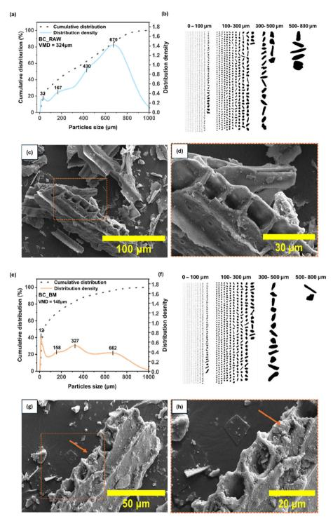
Fig. 1 Particle size and morphological characterization of biochar. Particle size distribution, DIA particle images and SEM micrographs of biochar (a–d) before (BC\_RAW) and (e–h) after ball milling (BC\_BM). In (g and h), the orange arrow indicates the collapsed pore structure.
