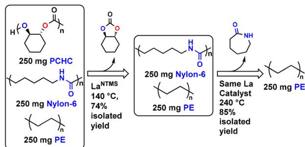
Scheme 2  $\text{La}^{\text{NTMS}}$  mediates the clean catalytic separation of PCHC + Nylon-6 + PE mixtures.
