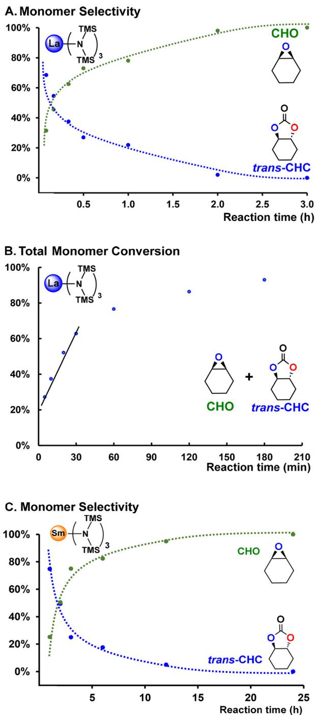
**Fig. 1** A. Kinetic profile of PCHC depolymerization in a closed reaction system using  $\text{La}^{\text{NTMS}}$  under the conditions of Table 1. B. Total monomer conversion (*trans*-CHC + CHO) versus reaction time. C. Kinetic profile of PCHC depolymerization in a closed reaction system using  $\text{Sm}^{\text{NTMS}}$ .
