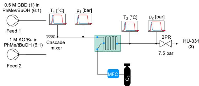
**Scheme 3** Continuous flow setup for the oxidation of CBD (1) to HU-331 (2). Conditions: Feed 1: 0.5 M CBD (1) in tBuOH/PhMe (6 : 1); Feed 2: 1 M KOtBu in tBuOH/PhMe with flow rates for Feed 1/Feed 2 = 2 : 2.1 mL min<sup>-1</sup>; 1.05 equiv. O<sub>2</sub> introduced through a mass flow controller. 7.5 bar backpressure was applied. The effluent was quenched into a vessel containing 0.5 M HCl.
