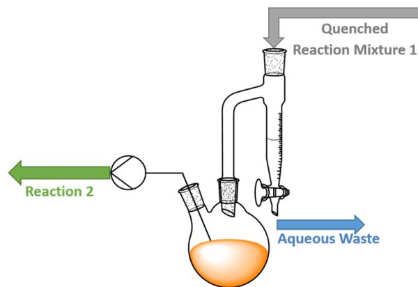
**Scheme 6** Continuous separation of phases using a Dean-Stark apparatus for telescoping the preparation Etrinabdione (**3**) from CBD (**1**).
