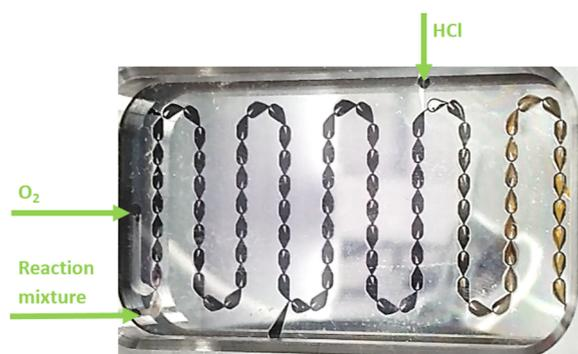
**Fig. 3** Image of the continuous flow oxidation of CBD (1) to HU-331 (2) with an inline quench by aqueous HCl solution. The first part of the reaction was a purple color. The color change from purple to orange indicated quenching of reactive intermediate 5.
