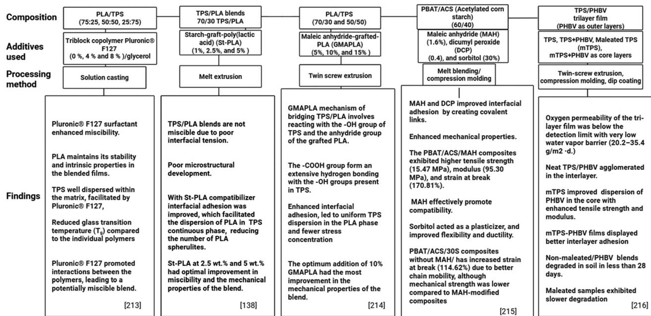
Fig. 8 Thermoplastic starch-based blends incorporating different additive and compatibilizers.<sup>138,213–216</sup>
