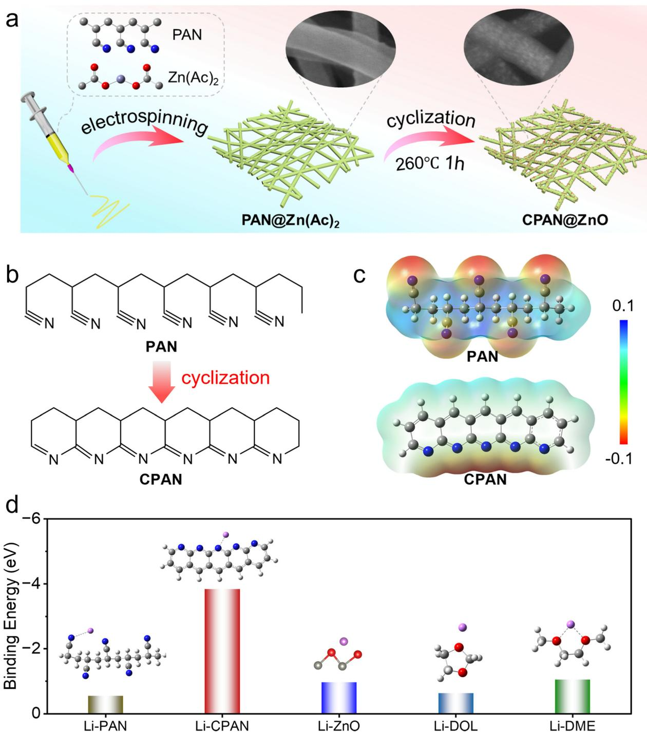
**Fig. 1** Design principles. (a) Schematic illustration of the synthesis process of CPAN@ZnO. (b) Schematic diagram of the cyclization reaction of PAN. (c) ESP. (d) Binding energies of Li-PAN, Li-CPAN, Li-ZnO, Li-DOL, and Li-DME.
