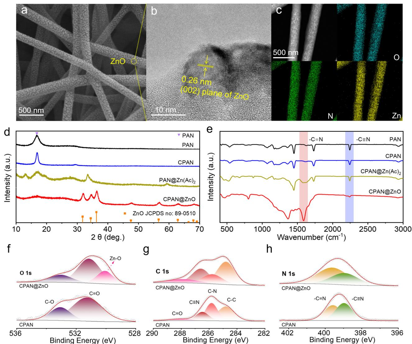
**Fig. 2** Micromorphology and chemical composition analysis. (a) SEM image. (b) High-resolution TEM image. (c) Elemental mapping of CPAN@ZnO. (d) XRD patterns before and after the cyclization reaction. (e) FT-IR spectra before and after the cyclization reaction, and analysis of the degree of cyclization with/without zinc ions. (f–h) High-resolution XPS spectra for O 1s, C 1s and N 1s of CPAN@ZnO and CPAN before cycling.
