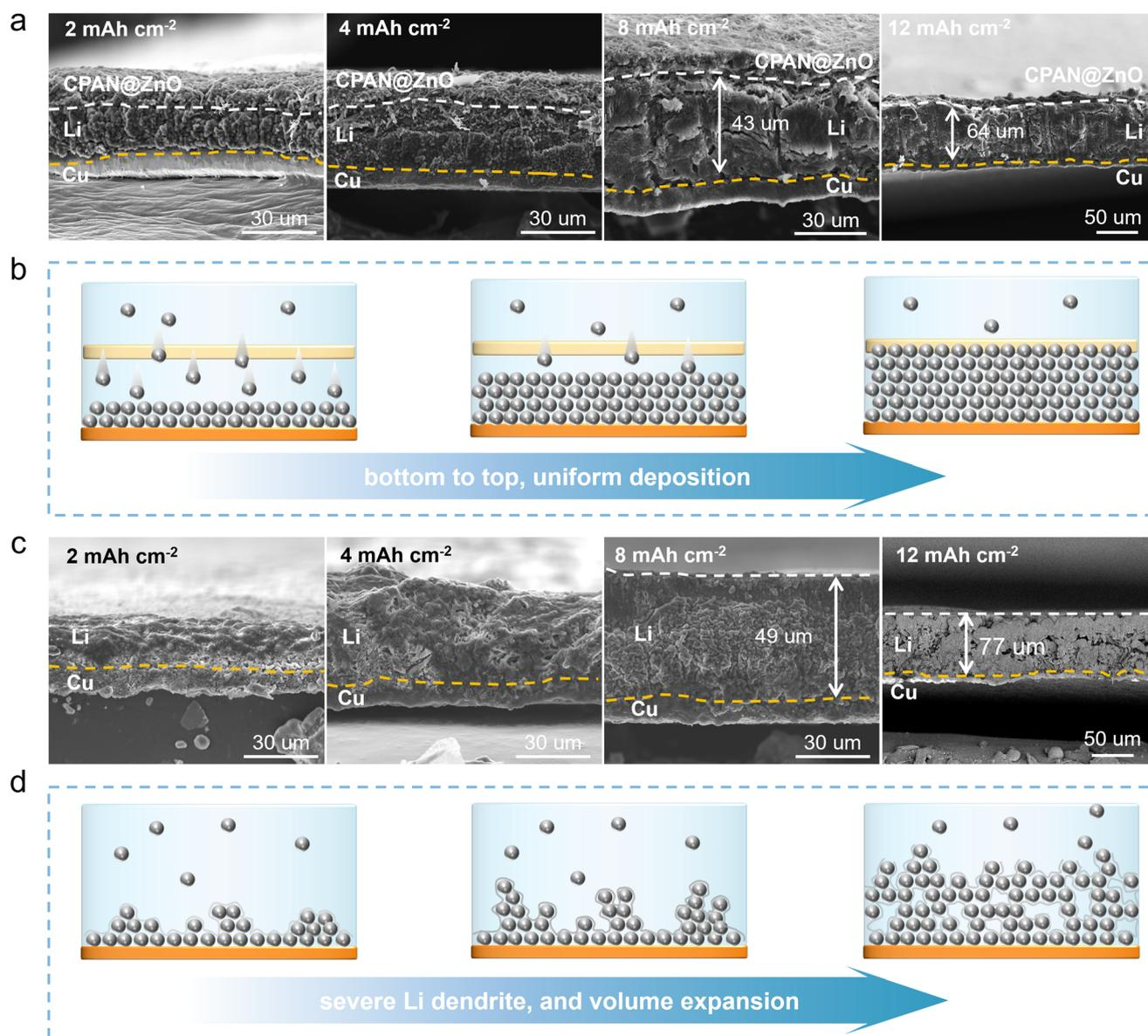
**Fig. 5** Li plating behaviours. (a and b) Li deposition behaviour on CPAN@ZnO@Cu. The SEM cross-section at different deposition capacities from 2 to 12 mA h cm<sup>-2</sup> and schematic diagrams of the corresponding deposition models. (c and d) Li deposition behaviour on bare Cu. The SEM cross-section at different deposition capacities from 2 to 12 mA h cm<sup>-2</sup> and schematic diagrams of the corresponding deposition models.
