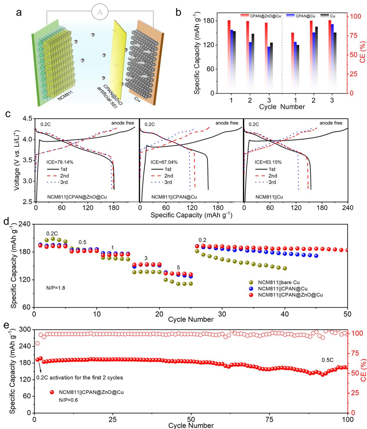
**Fig. 4** Electrochemical performance of full cells composed of NCM811 and CPAN@ZnO@Cu/CPAN@Cu/bare Cu. (a) Schematic of anode-free full batteries. (b and c) Comparison of specific capacity and CE for the first 3 cycles of anode-free batteries, and the corresponding charging/discharging curves. (d) Rate performance (the CPAN@ZnO@Cu, CPAN@Cu, and bare Cu anode are pre-lithiated, N/P = 1.8). (e) Cycling performance at 0.5 C of NCM811||CPAN@ZnO@Cu with an ultra-low N/P ratio of 0.6.
