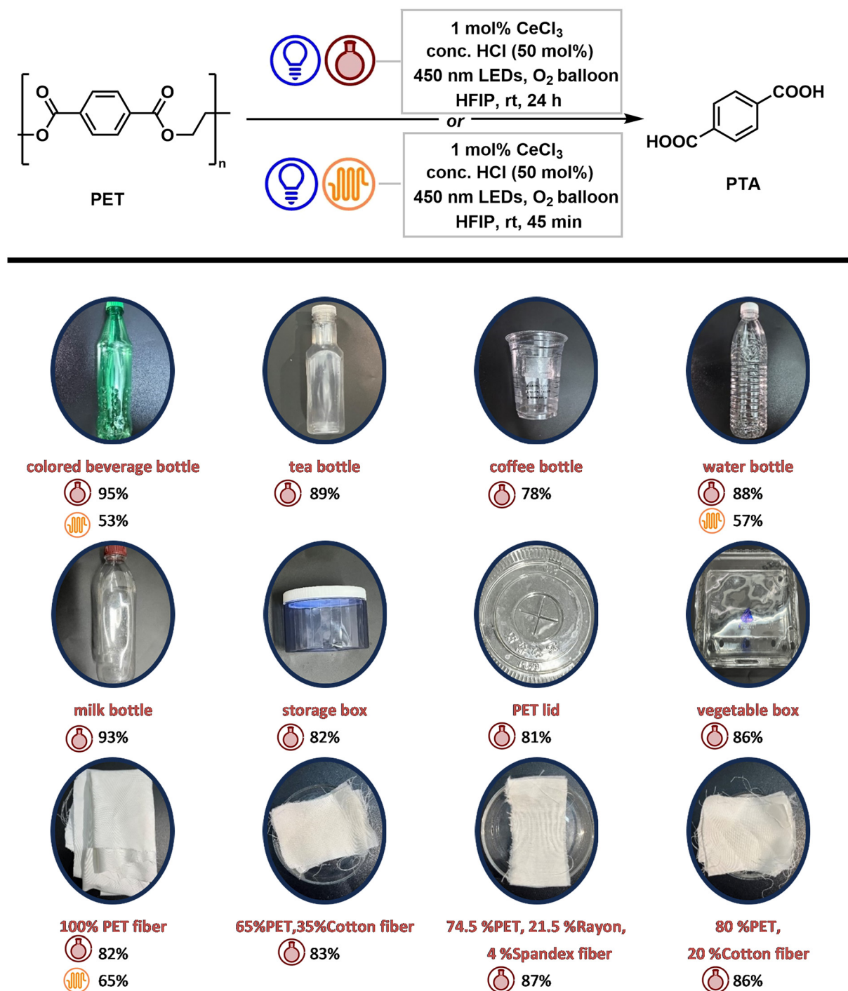
Fig. 2 Oxidative depolymerization of PET materials in batch a and flow b . a Polyester material (0.25 mmol, accounting for the repeat unit), CeCl 3 (1 mol%), HCl (50 mol%), HFIP (2.0 mL), 1 atm of O 2 , irradiation under 450 nm LEDs, 24 h, 25 °C. The yield was calculated based on isolation. b PET (0.5 mmol), CeCl 3 (1 mol%), conc. HCl (50 mol%), HFIP (10.0 mL) at room temperature (25 °C), blue LEDs (450 nm, 50 W), isolated yield.
