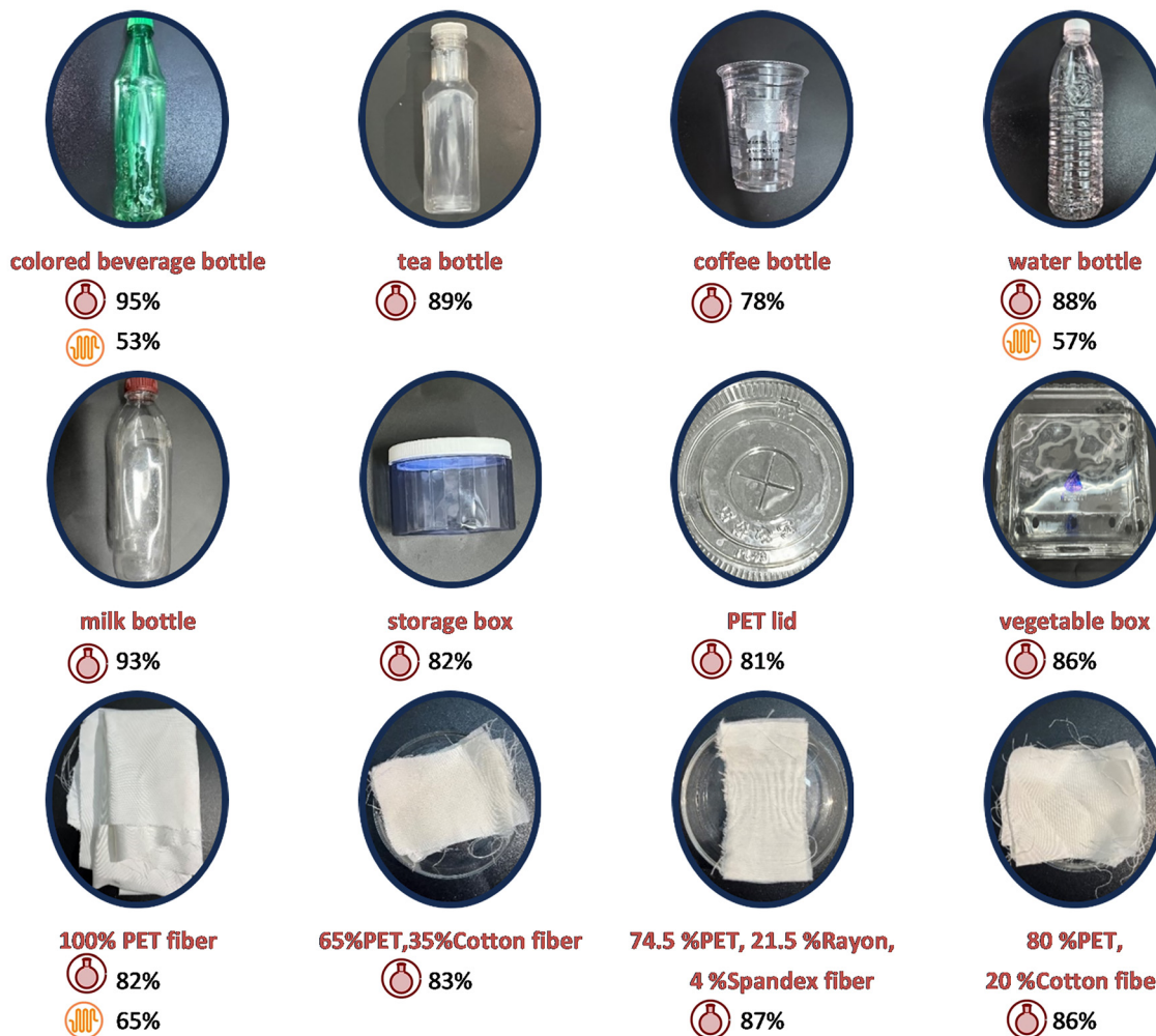
Fig. 2 Oxidative depolymerization of PET materials in batch a and flow b . a Polyester material (0.25 mmol, accounting for the repeat unit), CeCl 3 (1 mol%), HCl (50 mol%), HFIP (2.0 mL), 1 atm of O 2 , irradiation under 450 nm LEDs, 24 h, 25 °C. The yield was calculated based on isolation. b PET (0.5 mmol), CeCl 3 (1 mol%), conc. HCl (50 mol%), HFIP (10.0 mL) at room temperature (25 °C), blue LEDs (450 nm, 50 W), isolated yield.
