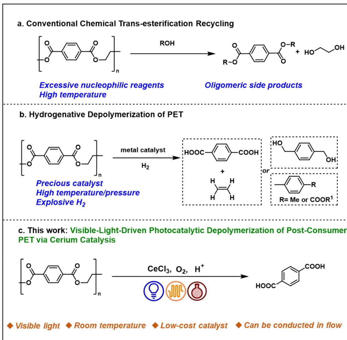
**Fig. 1** Polyethylene terephthalate recycling. (a) Chemical *trans*-esterification recycling. (b) Hydrogenative depolymerization of PET. (c) Visible-light-driven photocatalytic depolymerization of post-consumer PET via cerium catalysis.
