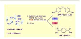
Scheme 3 Mixed stream PET/BPA-PC waste hydrolysis and selective precipitation.
