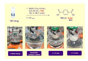
Scheme 2 Multigram scale PET (bottle) waste hydrolysis.
