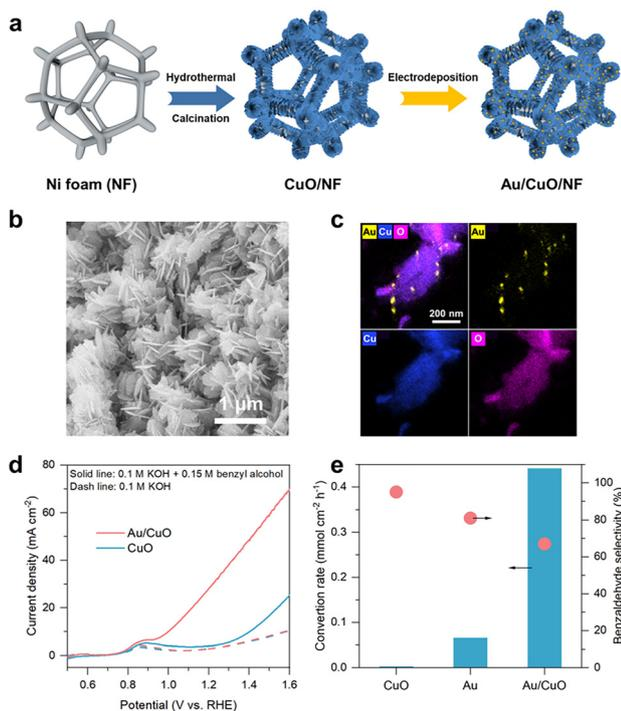
**Fig. 1** (a) Schematic illustration of the synthesis of the Au/CuO catalyst. (b) SEM image of Au/CuO. (c) STEM mapping of Au/CuO. (d) LSV curves in 0.1 M KOH (dashed line) and in 0.1 M KOH with 0.15 M benzyl alcohol (solid line) at a scan rate of  $10 \text{ mV s}^{-1}$  over different catalysts. (e) Conversion rate of benzyl alcohol and the corresponding selectivity for benzaldehyde at 1.16 V *vs.* RHE over different catalysts.
