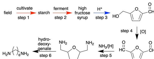
**Scheme 1** The synthesis of 1,6-hexanediamine from starch.<sup>7</sup>**Table 2** A convergent synthesis with one direct hotspot
