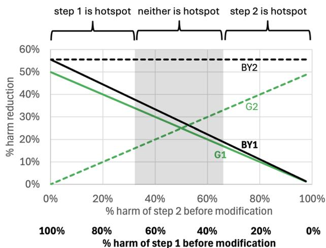
**Fig. 4** The % reduction in total harm per gram of product C that can be obtained for the reaction sequence in Scheme 2, where a large improvement in yield is possible. The assumptions are the same as those in Fig. 3 except that the BY1 and BY2 strategies increase the yield of either step 1 or step 2 by 125% (e.g. an initial yield of 40% changes to a yield of 90%). Thus  $y_i/y_i$  and  $z_i/z_i$  are 2.25 for BY1 and BY2, respectively.
