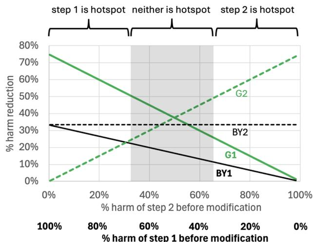
**Fig. 5** The % reduction in total harm that can be obtained for the reaction sequence in Scheme 2, where a large reduction in the harm of individual steps is possible. The assumptions are the same as those in Fig. 3 except that we assume the G strategy reduces the harm of an individual step by 75%.
