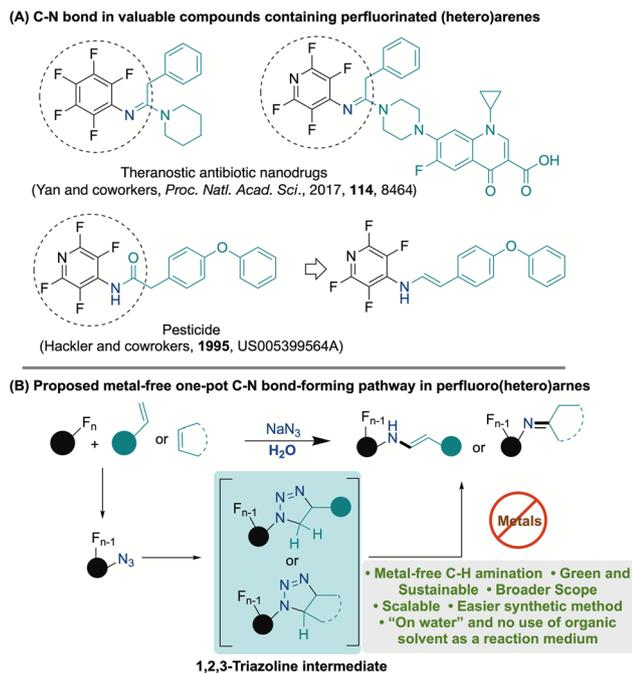
Fig. 1 "On water" metal-free C-H amination of perfluoroarenes.
