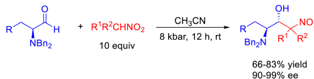
Scheme 9 Diastereoselective nitro–aldol reaction of \alpha -amino aldehydes with nitroalkanes under high pressure.
