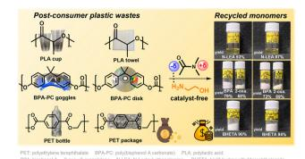
Scheme 1 Schematic illustration of this work: aminolytic degradation for chemical recycling of plastic wastes under mild and catalyst-free conditions.
