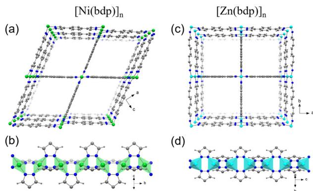
**Fig. 2** View along the pore channels and SBU chains in [Ni(bdp)]<sub>n</sub> (a and b)<sup>21,22</sup> and [Zn(bdp)]<sub>n</sub> (c and d). Solvent molecules and hydrogen atoms are not shown. C in grey, N in dark blue, Ni in green, and Zn in light blue.<sup>21,22,56</sup>
