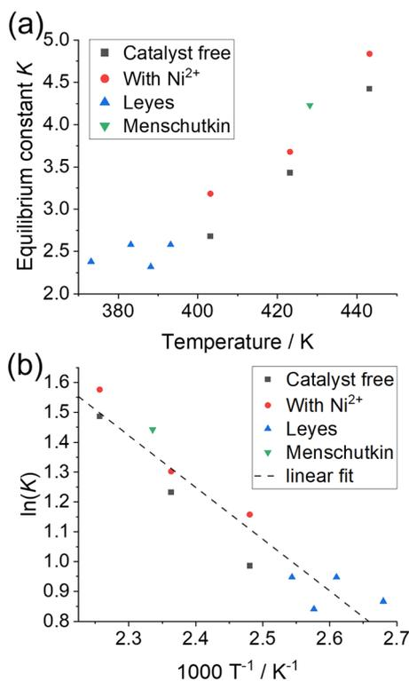
**Fig. 4** (a) Combined plots of published  $K$  values of the  $n$ -butyl acetate formation<sup>57,58</sup> and values from this study over the temperature in K. (b) Van 't Hoff plot of the equilibrium constant with linear fit over all values.
