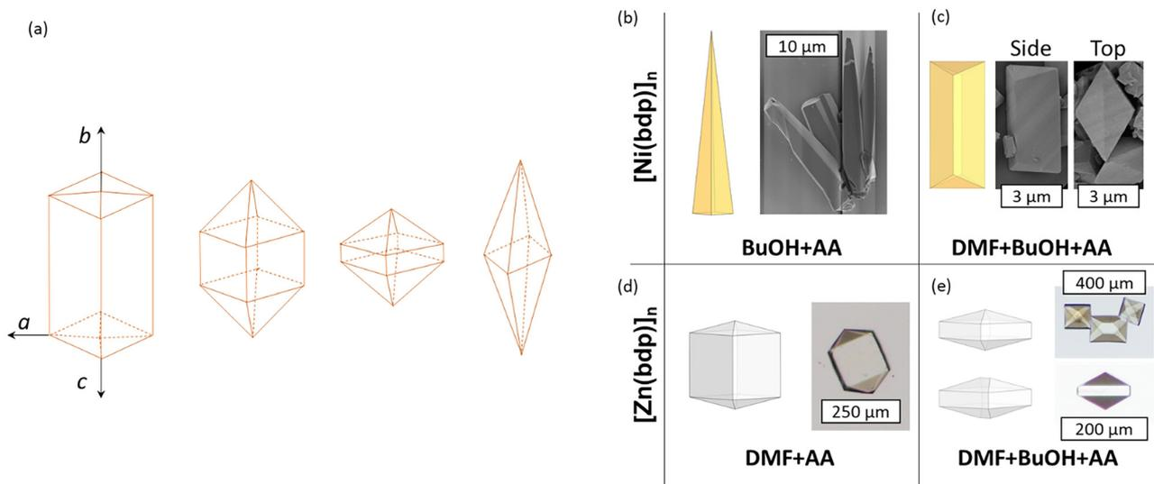
Fig. 9 (a) Shape evolution of the  $[\text{M}(\text{bdp})]_n$  crystals; (b–e) observed morphologies of  $[\text{Ni}(\text{bdp})]_n$  (a and b) and  $[\text{Zn}(\text{bdp})]_n$  (c and d) MOFs obtained from different solvent systems.
