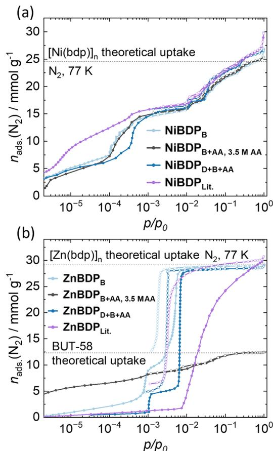
**Fig. 11** Nitrogen physisorption isotherms at 77 K represented in semi-logarithmic scale for (a)  $[\text{Ni}(\text{bdp})]_n$  and (b)  $[\text{Zn}(\text{bdp})]_n$  prepared by different synthesis methods and washed with NMP/DMF. Theoretical uptakes of the corresponding phases calculated using Mercury software<sup>87</sup> are indicated as dashed lines. Adsorption – filled symbols, desorption – open symbols.
