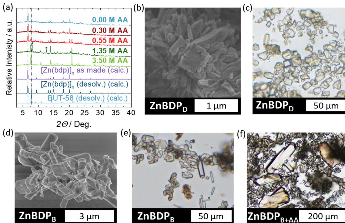
**Fig. 7** (a) PXRD patterns of the as-made  $\text{ZnBDP}_{\text{B}}$  and  $\text{ZnBDP}_{\text{B}+\text{AA}}$  synthesized with varying AA amounts in comparison to PXRD calculated from crystal structures of  $[\text{Zn}(\text{bdp})]_n$  (CCDC 2426284†) and BUT-58 (CCDC 2426285†); (b) SEM, (c) VLM images of  $\text{ZnBDP}_{\text{D}}$  (d) SEM, (e) VLM images of  $\text{ZnBDP}_{\text{B}}$  and (f) VLM image of  $\text{ZnBDP}_{\text{B}+\text{AA}}$ , 3.5 M AA.
