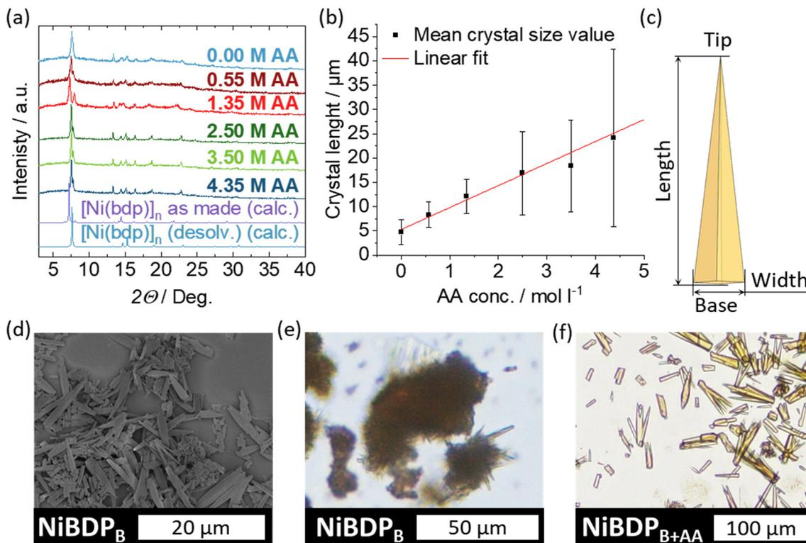
**Fig. 6** (a) PXRD patterns of the as-made **NiBDP<sub>B+AA</sub>** obtained with varying amounts of AA. (b) Increase in the average crystal length with the increasing amount of AA utilized. (c) Schematic representation of a typical **NiBDP<sub>B</sub>** or **NiBDP<sub>B+AA</sub>** crystal shape with descriptors. (d) SEM and (e) VLM images of **NiBDP<sub>B</sub>**. (f) VLM image of **NiBDP<sub>B+AA</sub>** obtained with 4.35 mol l<sup>-1</sup> of AA.
