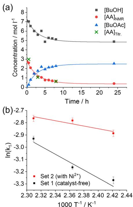
**Fig. 3** (a) Representative concentration profiles for the catalyst-free esterification reaction at 150 °C with numerical fits shown as solid lines; and (b) Arrhenius plots for catalyst-free and catalyzed reactions.
