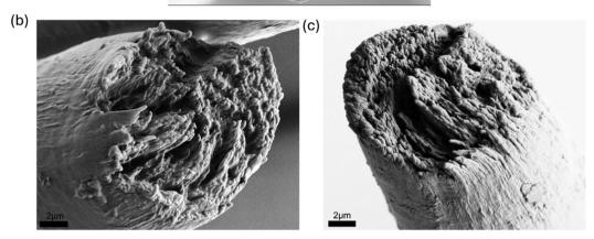
Fig. 2 Cross-sectional SEM images (5kX) of (a) Plain cellulose, MA-fibers (b) 40% MA, and (c) 50% MA.
