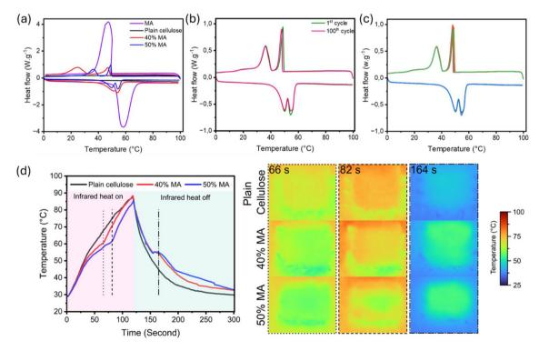
Fig. 3 DSC analysis of (a) all samples, (b) the 1<sup>st</sup> and 100<sup>th</sup> cycles of 50% MA, and (c) the entire 100 cycles. (d) The temperature profiles of textile samples with different PCM compositions over a 300 s duration (heater turned off at 120 s). The thermal images snapshots from the samples were taken at different time frames of 66 s, 82 s, and 164 s.
