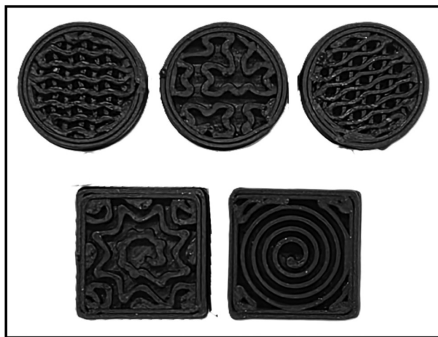
Fig. 2 Different infill pattern images from the PtNPs-G filament.
