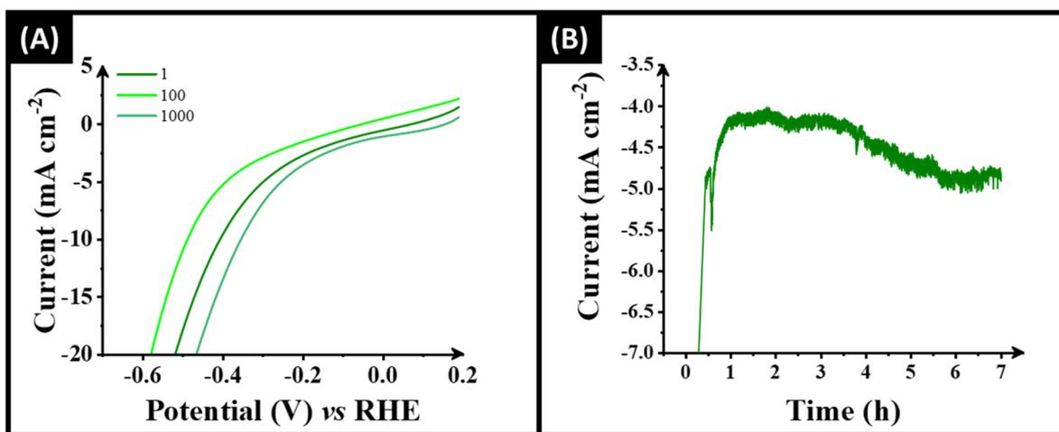
Fig. 5 Stability examination of PtNPs-G(12%) via (A) LSV (scan rate: 50 mV s<sup>-1</sup>) performed between the potential range of +0.2 to -0.6 V (vs. RHE), repeated for 1000 cycles. (B) Chronoamperometry for 7 hours at -0.30 V with PtNPs-G(12%) as WE (vs. RHE).
