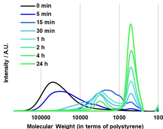
Fig. 4 Time-resolved GPC analysis of methanolysis reaction.
