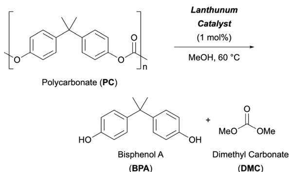
**Scheme 1** Methanolysis of PC with La complex catalyst.
