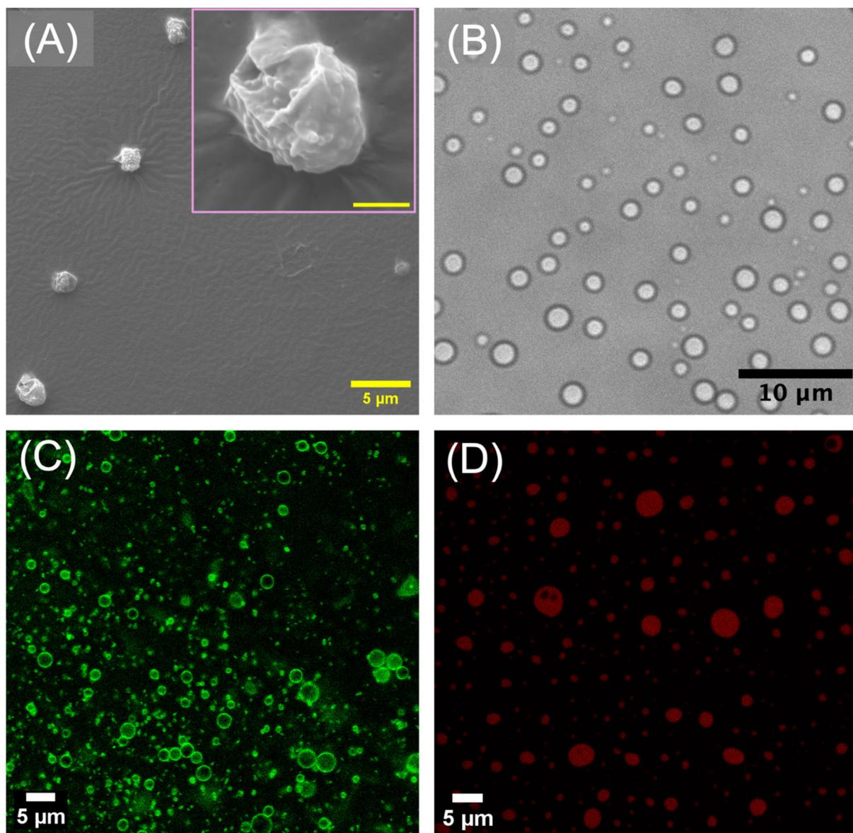
**Fig. 4** Characterization of microgelsomes prepared using PNSER microgels. (A) FE-SEM image of dried microgelsomes, with the inset image showing their collapsed morphology. (B) Optical image of microgelsomes prepared using a W/O emulsion droplet. CLSM images of interlinked microgelsomes prepared using (C) FITC-labelled PNSER microgels templated on the W/O emulsion droplet, and (D) PNSER microgels templated on the O/W emulsion droplet stained with hydrophobic Nile red (red fluorescent dye).
