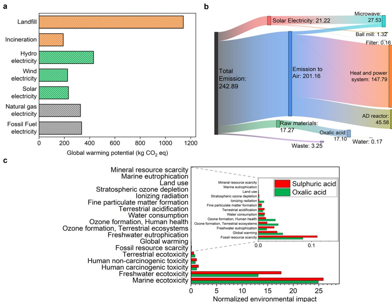
**Fig. 5** Life cycle assessment of the CBW processes: (a) GWP of the mechano-bio-thermochemical (MBTC) and conventional management processes (incineration and landfill). Electricity from renewable sources (hydro, wind, solar), natural gas and fossil fuel were considered in the CBW MBTC process. (b) Sankey diagram of our CBW process driven by solar electricity. (c) Normalized environmental impact score evaluation of sulphuric acid and oxalic acid when used in the CBW MBTC process.
