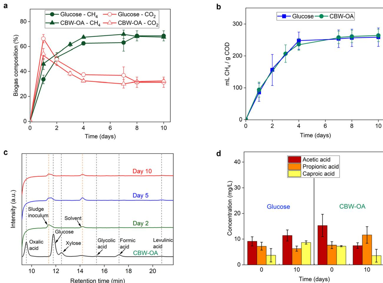
**Fig. 4** Methane production from cardboard waste (CBW) feed via anaerobic digestion over 10 days. Comparison of CBW-OA feed vs. glucose control with (a) biogas composition, and (b) cumulative methane production. (c) HPLC chromatogram: consumption of organic acids and sugars in CBW-OA feed. (d) Concentration of volatile fatty acids in CBW-OA and glucose feed.
