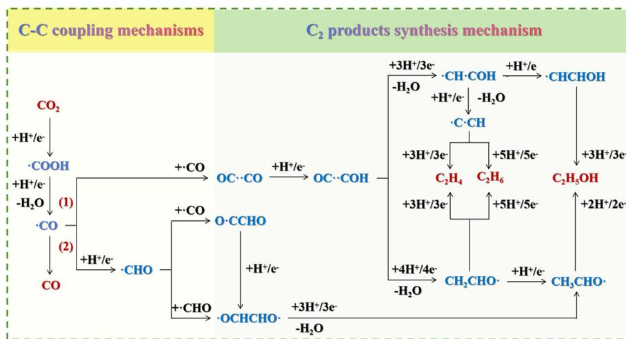
Fig. 6 Reaction pathways of CO<sub>2</sub> reduction to produce value-added C<sub>2</sub> chemicals (C<sub>2</sub>H<sub>4</sub>, C<sub>2</sub>H<sub>6</sub>, and C<sub>2</sub>H<sub>5</sub>OH) via electrocatalysis by adding (1) <sup>•</sup>CO before H<sup>+</sup>/e<sup>-</sup> and (2) H<sup>+</sup>/e<sup>-</sup> before <sup>•</sup>CO.
