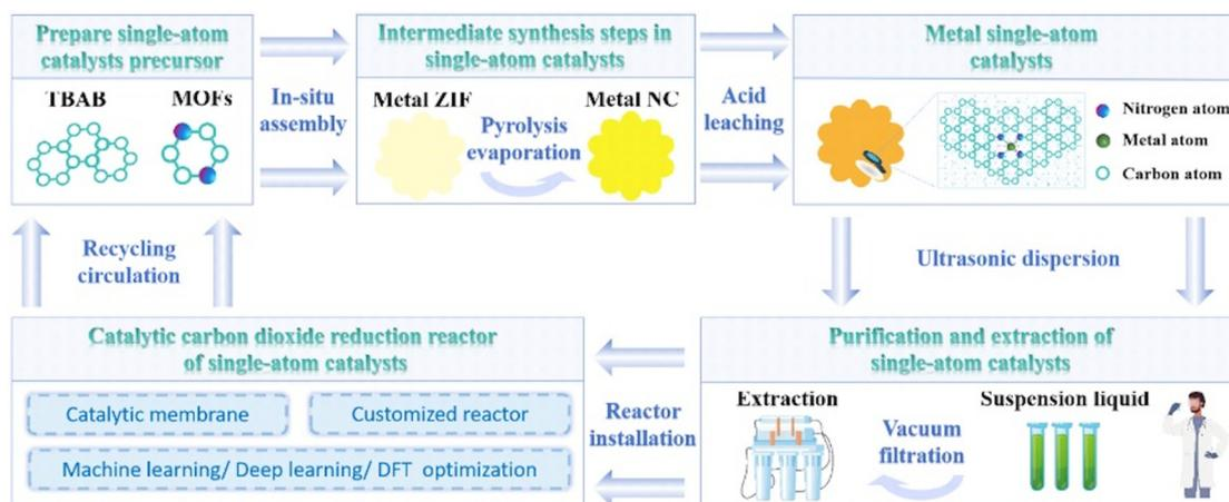
Fig. 3 Synthesis, purification, and application of single-atom catalysts for CO<sub>2</sub> reduction: from precursor preparation to catalytic reactor implementation.
