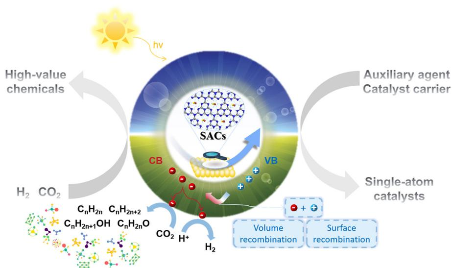
**Fig. 4** Engineering single-atom catalysts for efficient photocatalytic CO<sub>2</sub> reduction: modulation of the electron pair alignment and recombination dynamics using auxiliary agents and catalyst supports to enhance the catalyst stability.
