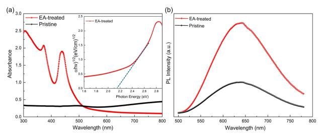
Fig. 7 (a) Absorption spectra measured by UV-vis-NIR spectroscopy for the ambient-processed pristine and EA-treated  $Cs_2AgBiBr_6$  films. Inset: Tauc plot of the indirect bandgap ambient-processed EA-treated  $Cs_2AgBiBr_6$  films. (b) Steady-state PL spectra for the ambient-processed pristine and EA-treated  $Cs_2AgBiBr_6$  films.
