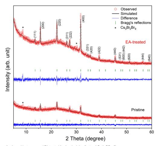
Fig. 5 XRD patterns for the ambient-processed EA-treated (top) and pristine (bottom) Cs<sub>2</sub>AgBiBr<sub>6</sub> films.
