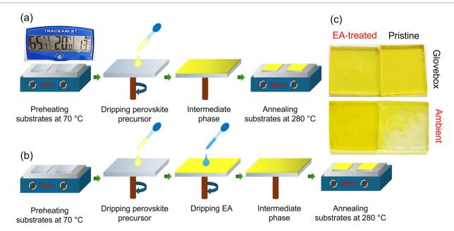
Fig. 1 (a) Schematic illustration of the ambient process to fabricate pristine  $Cs_2AgBiBr_6$  films with a humidity monitor showing an RH of 65.7% during the fabrication process. (b) Ambient process to fabricate EA-treated  $Cs_2AgBiBr_6$  films. (c) Photographic images of actual pristine and EA-treated  $Cs_2AgBiBr_6$  films coated on the FTO-glass fabricated in the ambient air and glovebox.
