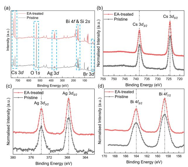
Fig. 6 (a) XPS survey spectra for the ambient-processed pristine and EA-treated  $Cs_2AgBiBr_6$  films. High-resolution XPS spectra of the element (b) Cs 3d, (c) Ag 3d, and (d) Bi 4f for the ambient-processed pristine and EA-treated  $Cs_2AgBiBr_6$  films.
