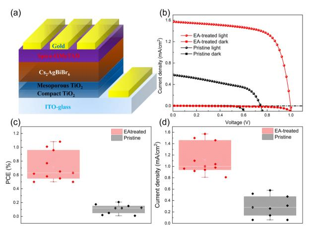
Fig. 8 (a) Schematic representation of PSCs based on ITO-glass/compact and mesoporous  $TiO_2/Cs_2AgBiBr_6/spiro-OMeTAD/Au$  architecture. (b) J-V curves under AM1.5 sunlight and dark for champion cells based on the ambient-processed pristine and EA-treated films. (c) PCE and (d)  $J_{SC}$  distribution for the PSCs based on the ambient-processed pristine and EA-treated films.
