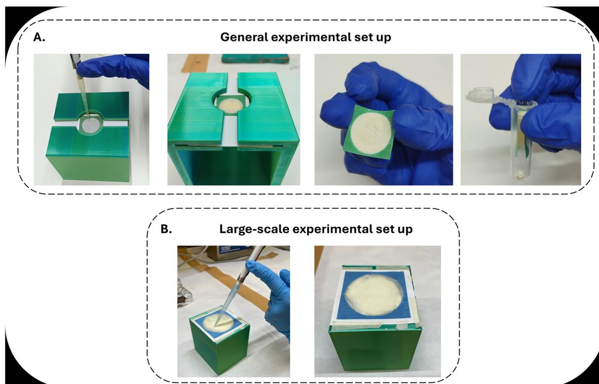
**Fig. 2** Images of (A) the experimental setup for the general procedure, *i.e.*, 0.14 mmol scale and the (B) large-scale, *i.e.*, 1.4 mmol scale, experimental setup. The filter paper disc diameter is scalable to (A) 2 cm or (B) 6 cm according to the experimental needs. A 3D-printed device was employed as a housing for the paper-based platform to ensure stability throughout the entire procedure (from mixing of reagents to drying in a fume hood).
