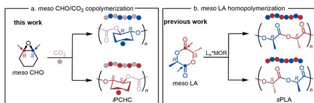
**Scheme 1** *Meso*-desymmetrization catalysis in the ROCOP of CHO and CO<sub>2</sub> (a) and in the ROP of *meso*-LA (b).
