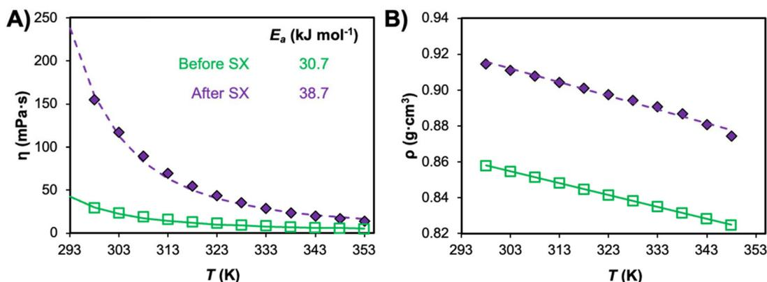
Fig. 9 Evolution in the (A) viscosity and (B) density of the TOPO + decanoic acid system ( $x_{\text{TOPO}} = 0.5$ ) as prepared (before SX) and after metal ion loading (Co<sup>2+</sup> and Mn<sup>2+</sup> mixture) of 44 g L<sup>-1</sup> in the DES phase; data are taken from refs. 47 and 131. The activation energy of viscous flow ( $E_a$ ) was also calculated from the viscosity data and provided in the inset.
