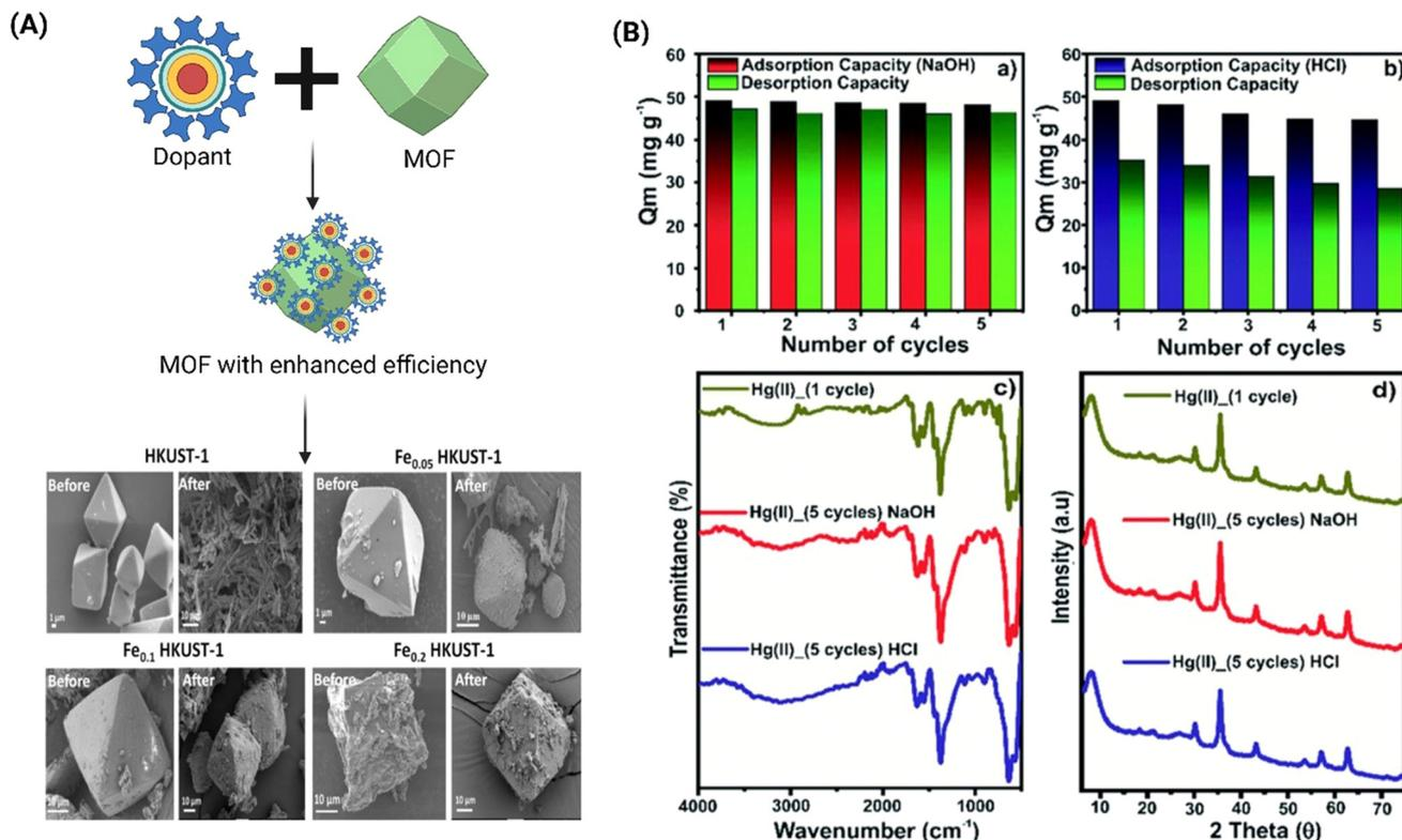
**Fig. 2** Strength of MOFs (A) doping of MOFs improves their efficiency. (F) SEM images show that doping of HKUST-1 MOFs with Fe ions improved its hydrolytic stability.<sup>21</sup> (B) The Zr-MOF@Fe<sub>3</sub>O<sub>4</sub> composite shows high adsorption capacity with only a slight reduction over 5 cycles<sup>22</sup>. (Prepared using Biorender Software).
