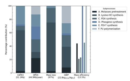
Fig. 13 Percentage contribution of each subprocess to the bio-PU production process across five key parameters: CAPEX, OPEX, mass loss, GWP, and mass efficiency. The total values for each parameter are indicated in the x-axis labels.
