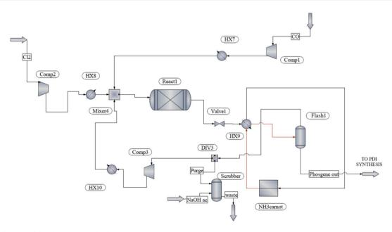
Fig. 5 Flow diagram of the phosgene synthesis process.
