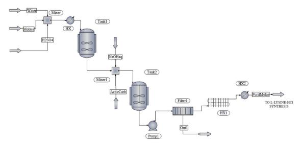
Fig. 2 Flow diagram of sugarcane molasses pretreatment.
