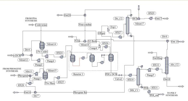
Fig. 6 Flow diagram for PDA phosgenation to produce pentamethylene diisocyanate (PDI).
