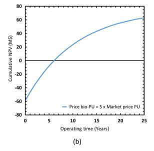
Fig. 9 Economic performance of the plant: (a) annual gross profit generated with different selling price ratios for the bio-PU with respect to the current market price for the fossil-based PU gel (ac. 3000 \$ per ton); (b) cumulative net present value during the estimated lifetime for the processing plant.
