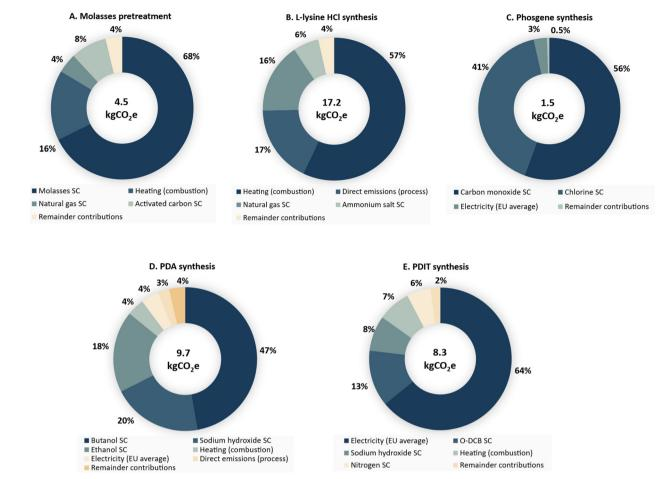
Fig. 12 Contribution of each subprocess to the total carbon footprint of 1 kg of the bio-PDI-T prepolymer produced with a cradle-to-gate perspective. Values are compiled in the ESI (Tables S9–S14†).
