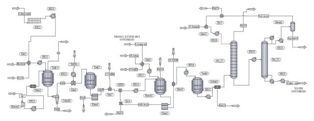
Flow diagram for the production of 1,5-pentanediamine (cadaverine) hydrochloride via the decarboxylation of L-lysine hydrochloride.
