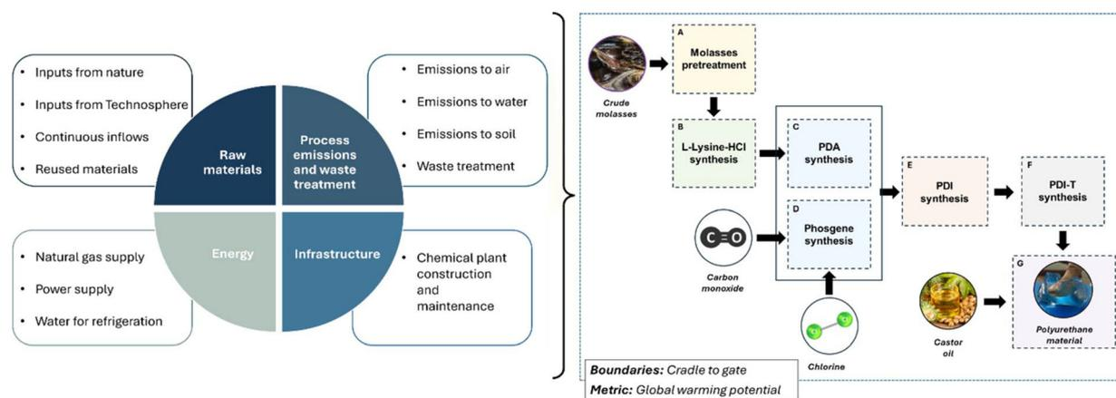
Fig. 8 Life-cycle assessment inventory construction and system boundaries of the biogenic polyurethane production supply chain.
