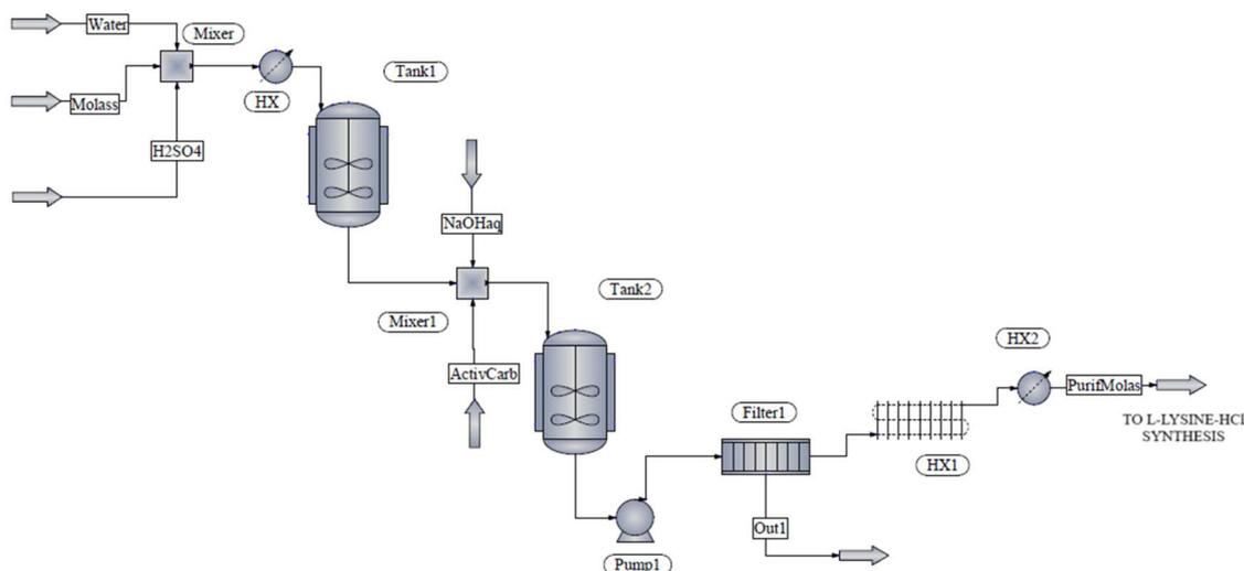
Fig. 2 Flow diagram of sugarcane molasses pretreatment.
