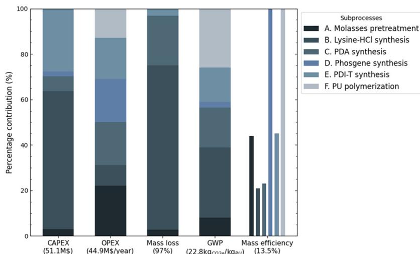
**Fig. 13** Percentage contribution of each subprocess to the bio-PU production process across five key parameters: CAPEX, OPEX, mass loss, GWP, and mass efficiency. The total values for each parameter are indicated in the x-axis labels.
