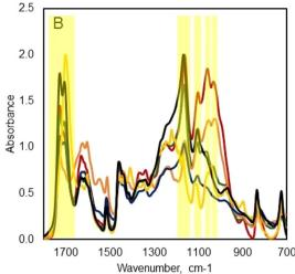
Fig. 6 FTIR spectrum of raw tomato peel (orange), ext free TP acid hydrolysis (blue), ext free TP alkaline hydrolysis (yellow), reference cutin (black), product 0.48 s (red), and product 1.51 s (green) in the range of wavenumber  $2800-3700 \text{ cm}^{-1}$  (A) and  $700-1800 \text{ cm}^{-1}$  (B).
