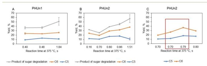
Fig. 11 The yield of C5, C6, and product of sugar degradation for experiments done on PhUN1 (A), on PhUN2 (B) and comparison of yields for experiments without and with the addition of acetic acid-framed (C).
