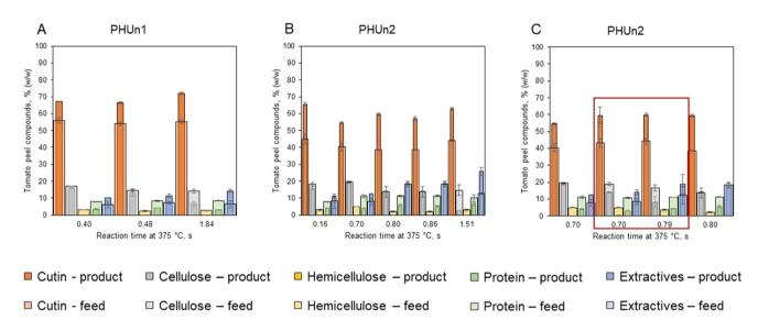
Fig. 4 Solid product composition and feed composition over different reaction times at 375 °C for experiments done on PhUN1 (A), on PhUN2 (B) and comparison of experiments without and with the addition of acetic acid – framed (C).
