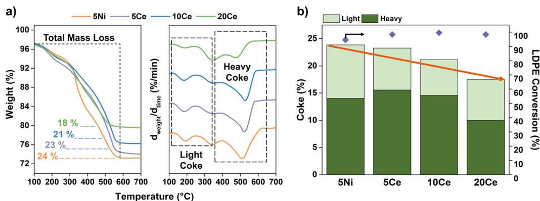
Fig. 4 TGA thermograms of (a) weight loss (%) and derivative weight loss (% min<sup>-1</sup>) and (b) light/heavy coke content comparison for the spent 5Ni/BEA (5Ni) and Ce-promoted 5Ni%Ce/BEA (%Ce = 0, 5, 10, 20) catalysts after 3.5 h hydrocracking reaction (2 g LDPE, 0.025 g catalyst, 300 °C, 30 bar).
