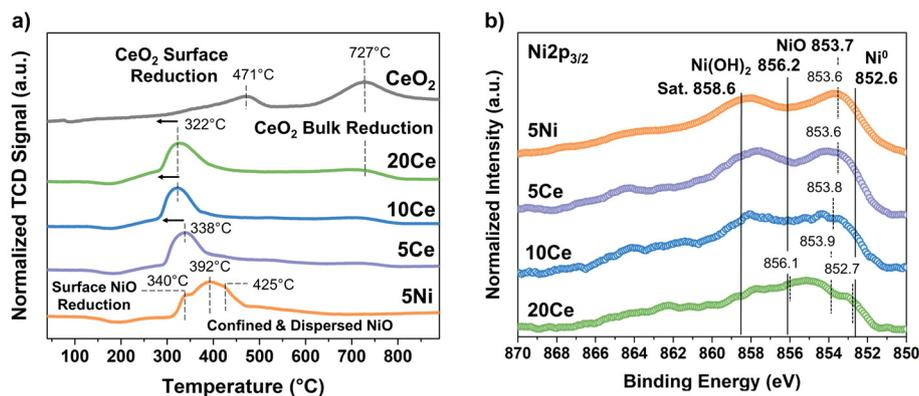
Fig. 3 Characterization of 5Ni%Ce/BEA (%Ce = 0, 5, 10, 20) catalysts: 5Ni (orange), 5Ce (purple), 10Ce (blue), and 20Ce (green). (a) H<sub>2</sub>-TPR profiles. (b) Air-free XPS spectra of the Ni 3p<sub>3/2</sub> region normalized to C 1s at 284.8 eV.
