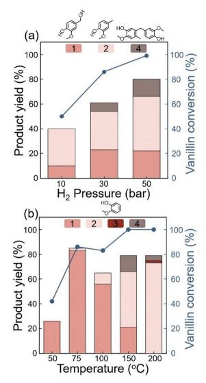
Fig. 4 Effects of (a)  $\rm H_2$  pressure measured at room temperature and (b) reaction temperature exhibiting products of VANOL (1), CRSOL (2), and dimer 1 (4). (Reaction conditions: 2 mmol of VAN in a mixed solvent of 30 mL of DI water and 15 mL of n-octane, 50–200 °C of reaction temperature, 1 h of reaction time, 0.05 g of 1 wt% Ru/C catalyst, catalyst/substrate = 0.17 w/w, 10–50 bar of  $\rm H_2$  pressure measured at room temperature.)
