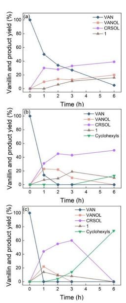
Fig. 5 Effects of reaction pressure and time on VAN hydrogenation and condensation for (a) 10 bar, (b) 30 bar, and (c) 50 bar of  $\rm H_2$  pressure measured at room temperature. (Reaction conditions: 2 mmol of VAN in a mixed solvent of 30 mL of DI water and 15 mL of n-octane, 0.05 g of 1 wt% Ru/C catalyst, 150 °C of reaction temperature.)
