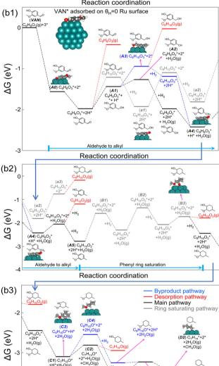
**Fig. 7** Energy diagram of VAN adsorbed on Ru surface covered with (a) 1 ML H\* and (b1, b2 and b3) 0 ML H\*. (p) denotes a physisorbed molecule.
