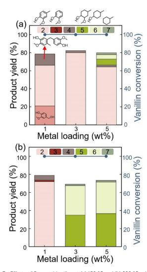
Fig. 3 Effects of Ru metal loading at (a) 150 °C and (b) 200 °C exhibiting products of CRSOL (2), GUA (3), dimer 1 (4), 2-methoxy-4-methylcyclohexanol (5), 4-methyl cyclohexanol (6), methyl cyclohexane (7). (Reaction conditions: 1–5 wt% Ru/C catalysts, 2 mmol of VAN in a mixed solvent of 30 mL of DI water and 15 mL of n-octane, 1 h of reaction time, 0.05 g of Ru/C catalyst, 50 bar of  $H_2$  pressure measured at room temperature.)
