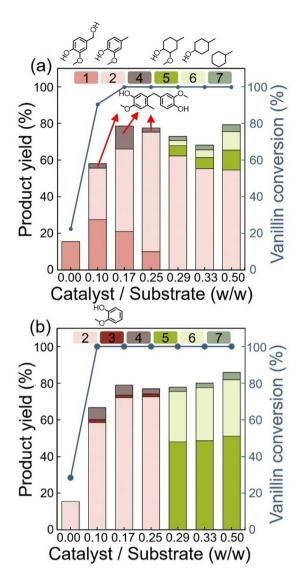
Fig. 1 Effects of catalyst-to-substrate ratio at (a) 150 °C and (b) 200 °C exhibiting products of CRSOL (2), GUA (3), dimer 1 (4), 2-methoxy-4-methyl-cyclohexanol (5), 4-methyl cyclohexanol (6), methylcyclohexano (7). (Reaction conditions: 2 mmol of VAN, a mixed solvent of 30 mL of DI water and 15 mL of n-octane, 1 h of reaction time, 0.03–0.15 g of 1 wt% Ru/C, 50 bar of H $_2$  pressure measured at room temperature.)
