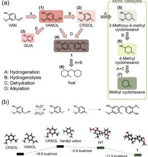
Fig. 8 (a) Reaction pathway of hydrogenation and condensation of VAN using Ru/C and (b) its energy profile for the condensation of VANOL and CRSOL through the formation of intermediate (INT).
