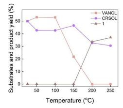
Fig. 6 Product compositions of non-catalytic condensation of VANOL and CRSOL. Reaction conditions: 1 mmol of VANOL and CRSOL each, 30 mL of DI water, 15 mL of n-octane, 50 bar of  $N_2$  pressure (measured at room temperature), 3 h of reaction time.
