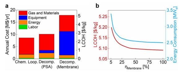
Fig. 7 (a) Annual cost and levelized cost of hydrogen (LCOH) for CLAOD-WS and for CAD equipped with pressure swing absorption (PSA) or Pd-Ag/ceramic membrane separation. (b) Dependence of LCOH and total system energy consumption rate on H<sub>2</sub> separation membrane Second Law efficiency in CAD process with Pd-Ag/ceramic membrane separation.
