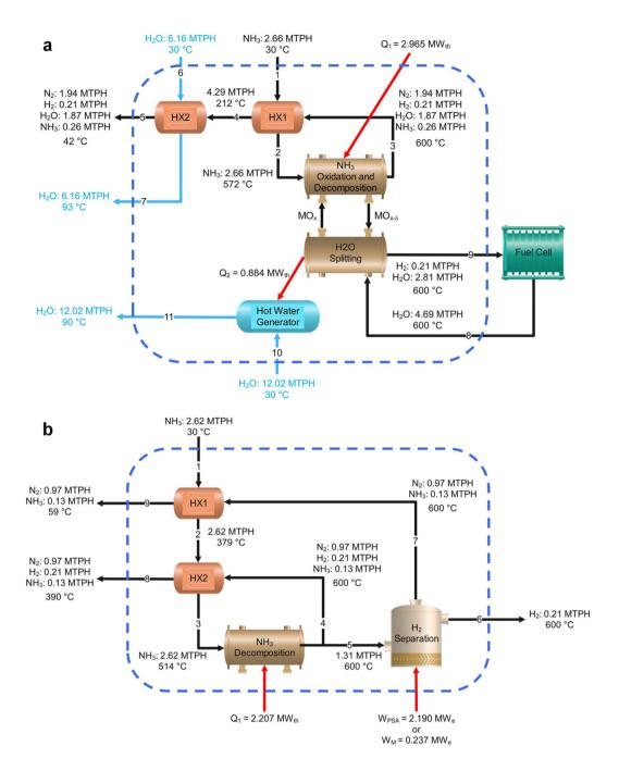
Fig. 6 Process schematics with major model parameters of (a) chemical looping ammonia oxidation and decomposition integrated with water splitting (CLAOD-WS), and (b) catalytic ammonia decomposition (CAD). MTPH: metric ton per hour.
