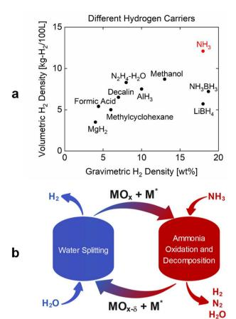
Fig. 1 (a) Comparison among chemical hydrogen carriers for volumetric and gravimetric hydrogen densities at 0.1 MPa and 240 K. Adapted from references.  $^{1,12,13,17-20}$  (b) Chemical looping ammonia oxidation and decomposition integrated with water splitting (CLAOD-WS) process schematic.  $MO_x$  is a redox active metal oxide, and M\* is a metallic catalyst. Compositions of M and M\* may change between the reduced and oxidized states.
