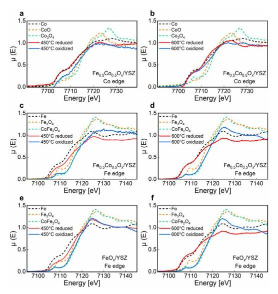
Fig. 5 Simultaneous redox reactions of Fe and Co for CLAOD-WS. XANES results for Co and Fe between NH<sub>3</sub>-reduced and steam-oxidized states: Co K edge of Fe<sub>0.5</sub>Co<sub>0.5</sub>O<sub>x</sub>/YSZ at (a) 450 °C and (b) 600 °C, Fe K edge of Fe<sub>0.5</sub>Co<sub>0.5</sub>O<sub>x</sub>/YSZ at (c) 450 °C and (d) 600 °C, and Fe K edge of FeO<sub>x</sub>/YSZ at (e) 450 °C and (f) 600 °C.
