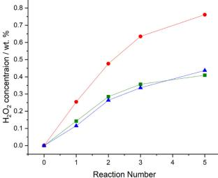
Fig. 7 Comparison of catalytic activity over sequential H<sub>2</sub>O<sub>2</sub> synthesis reactions. Key: 0.5%Au-0.5%Pd/TiO<sub>2</sub> (green squares), 0.5%Au-0.5%Pd-0.02%Fe/TiO2 (red circles), and 0.5%Au-0.5%Pd-1.0%Fe/TiO2 (blue triangles). H<sub>2</sub>O<sub>2</sub> direct synthesis reaction conditions: catalyst (0.01 g), H<sub>2</sub>O (2.9 g), MeOH (5.6 g), 5% H<sub>2</sub>/CO<sub>2</sub> (420 psi), 25% O<sub>2</sub>/CO<sub>2</sub> (160 psi), 0.5 h, 2 °C, 1200 rpm.
