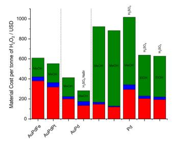
Fig. 8 Techno-economic analysis of the direct synthesis of H<sub>2</sub>O<sub>2</sub> over the optimal AuPdFe/TiO<sub>2</sub> catalysts and comparison to alternative formulations. Key: H2 (red bar), catalyst (blue bar) and organic component of reaction solvent (green bar, ethanol or methanol as indicated), promoters utilised as indicated. Additional data is provided in Tables S7A-J.†
