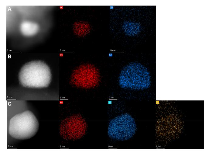
Fig. 4 Representative HAADF-STEM micrographs and complementary EDX analysis of individual alloy nanoparticles in (A) 0.5%Au-0.5%Pd/TiO<sub>2</sub>, (B) 0.5%Au-0.5%Pd-0.02%Fe/TiO2 and (C) 0.5%Au-0.5%Pd-1%Fe/TiO2. Note: catalysts exposed to a reductive heat treatment prior to use (5%H2/Ar, 400 °C, 4 h, 10 °C min<sup>-1</sup>).
