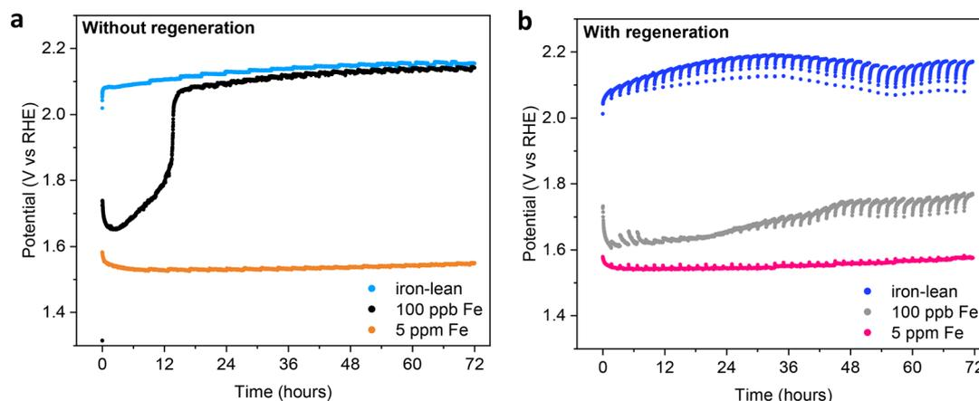
**Fig. 3** Chronopotentiometry at 300 mA cm<sup>-2</sup> for 72 h at 30 °C of nickel wire electrodes without (a) and with (b) regeneration, in an iron-lean electrolyte, iron-lean electrolyte with 100 ppb Fe intentionally added (to mimic the iron content of a commercial 1.0 M KOH electrolyte), and iron-rich electrolyte (5 ppm Fe). The potential is *iR* compensated.
