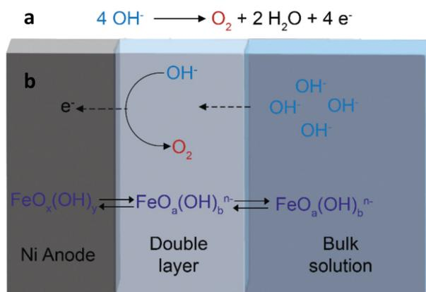
**Fig. 1** (a) The oxygen evolution reaction (OER) occurring at the anode of a water electrolyser in an alkaline environment. (b) Schematic representation of the main mass transfer phenomena involving dissolution/redeposition of iron species stemming from the electrolyte, occurring during the OER on a Ni electrode.
