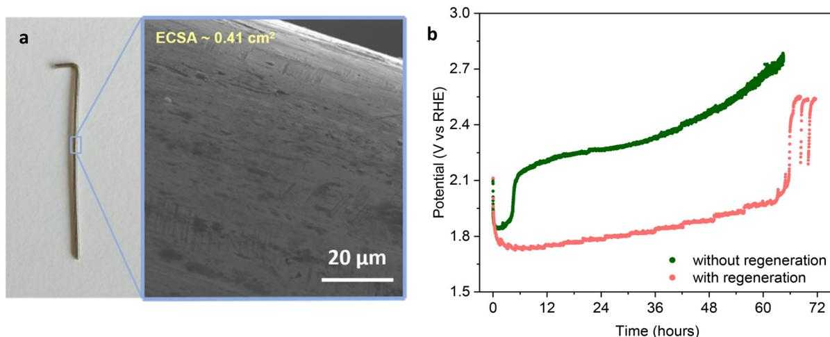
**Fig. 6** (a) A fresh nickel wire and a SEM image of its surface. (b) Chronopotentiometry at  $800 \text{ mA cm}^{-2}$  for 72 h of bare nickel electrodes with and without regeneration, with 120 ppb Fe added to an iron-lean 1.0 M KOH electrolyte. The experiments were carried out at  $30^\circ\text{C}$ . The potential is reported vs. RHE and it is  $iR$  compensated. The regeneration steps were performed by lowering the applied potential to 1.43 V for 100 s every 100 min of electrolysis.
